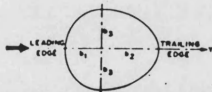
Figure 6.8 Elliptical cross-section as simplification of distorted jet (31).
