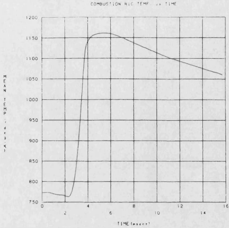
Figure 5.5 Mean chamber temperature produced from heat release analysis. Test 182
