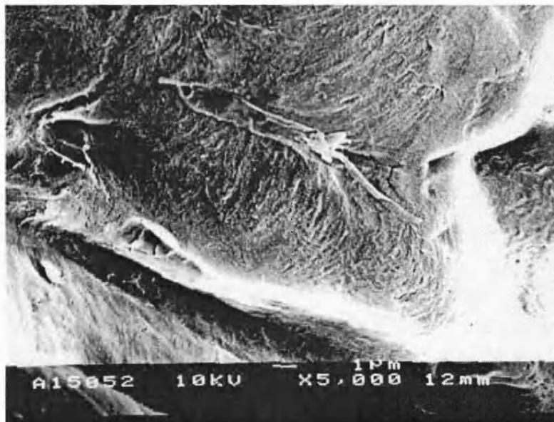
Figure 115: PE/PP (8), Sonicated with pressure 20x3.5s, 240 0 C, mag x5,000
