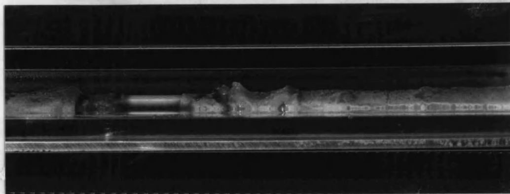
Figure 5.69(e): Photograph of wheat starch deposit contacted with 0.01 wt% Synperonic LF/CS 1000 + 0.5 wt% NaOH at 50°C and 4 l/min for 20 minutes.
