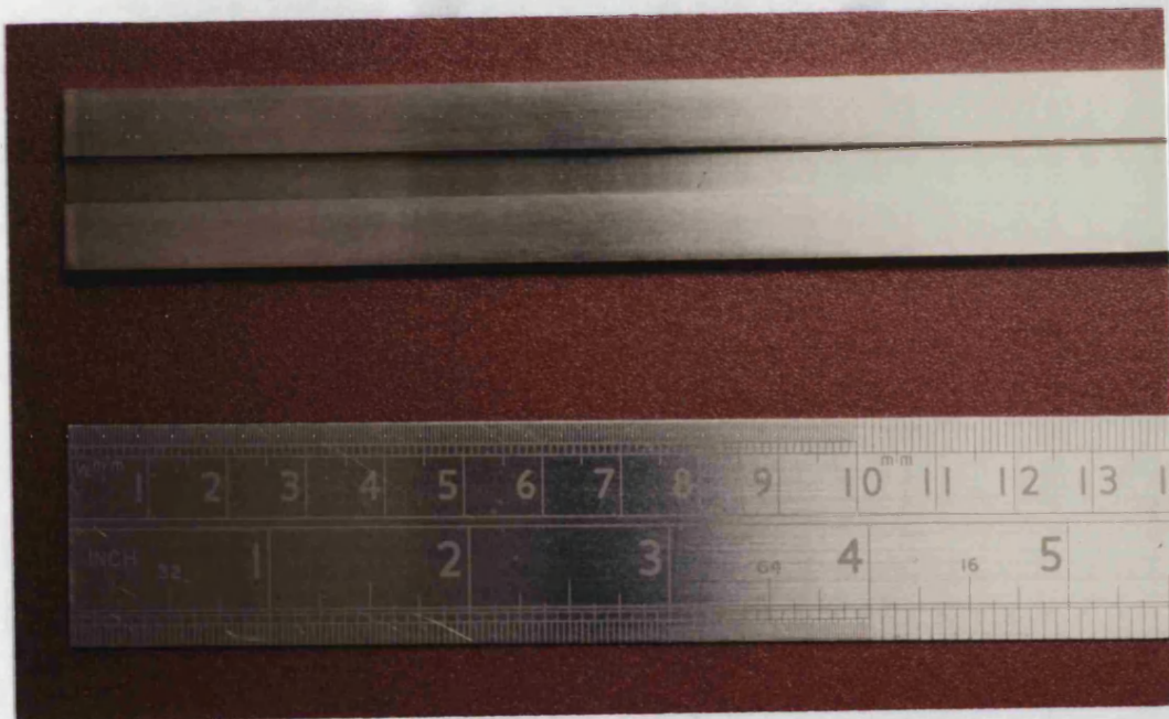
Figure 4.6(b) Top view photograph of test-plate fabricated with a 2 mm depth groove
