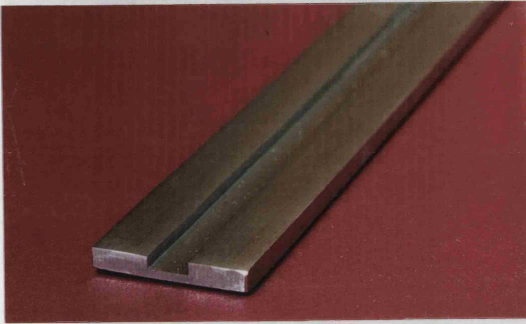
Figure 4.6(c) Side view photograph of test-plate fabricated with a 2 mm depth groove.
