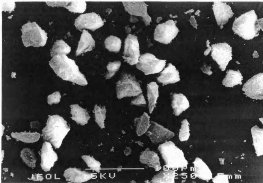
Figure 3.1.12. SEM micrograph showing a typical selection of particles from powder XPT W 601, mag. \times 250 .
