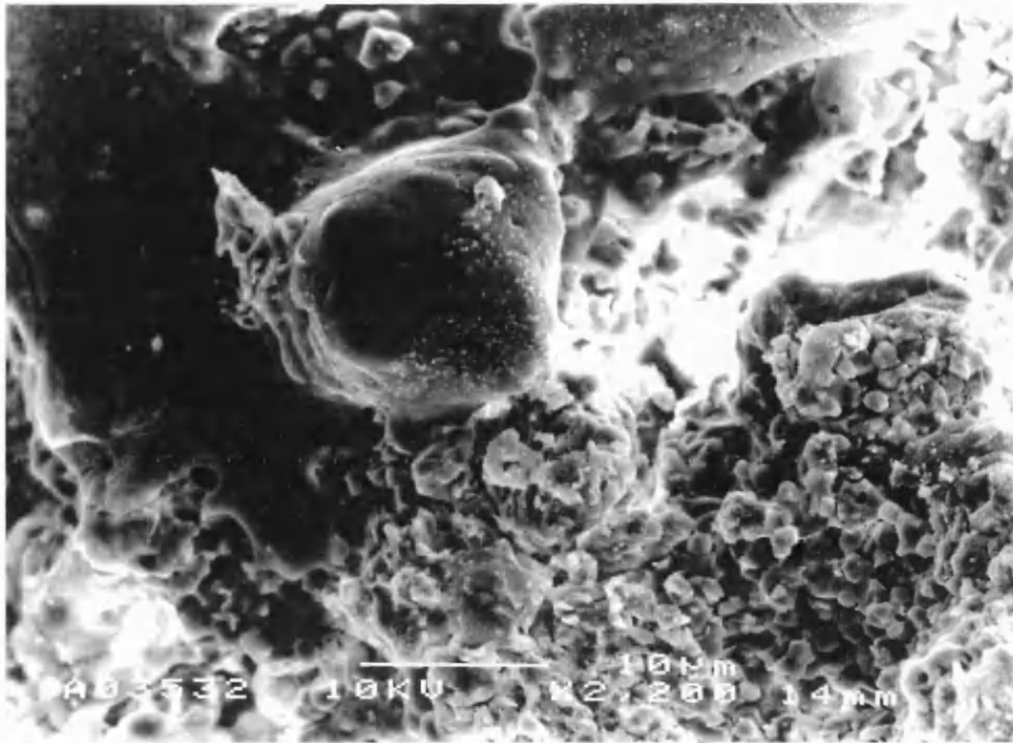
Figure 3.7.31. SEM micrograph of the HA coating APS3 aged for 1 week at pH4.5, showing etched and unetched areas. mag. \times 2200 .
