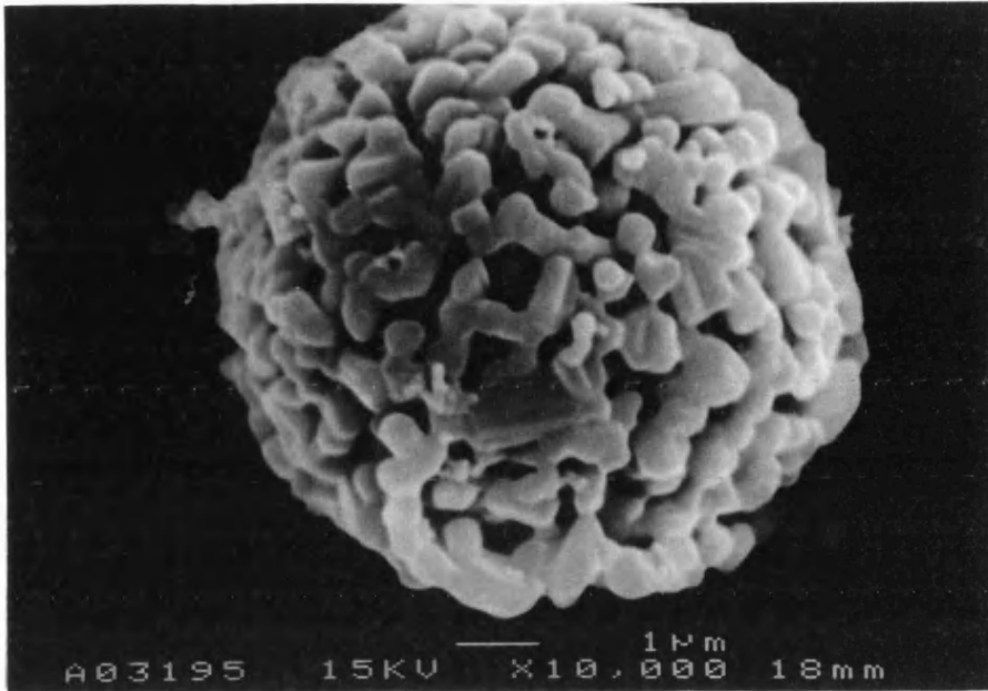
Figure 3.1.11. SEM micrograph showing a spherical particle of powder HA 044, mag \times 10000 .
