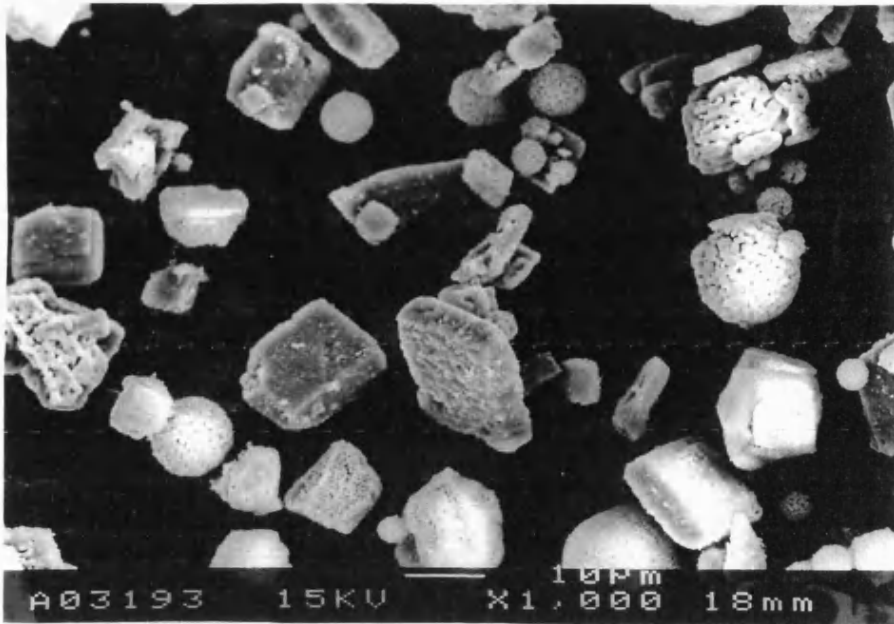
Figure 3.1.9. SEM micrograph showing a typical selection of particles from powder HA 044, mag. \times 1000 .
