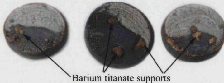
Figure 5.65: The under side of the BaTiO 3 -5.7wt% platinum samples indicating the barium titanate supports and the composite colour change to grey/white on contact with the alumina base plate. Discs are approximately 12 mm in diameter.
