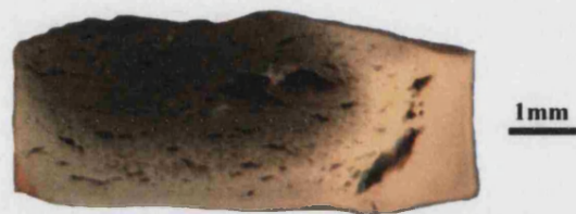
Figure 5.46: Large void formation due to gas generation in BaTiO 3 -2wt% silicon carbide sintered at 1350°C.
