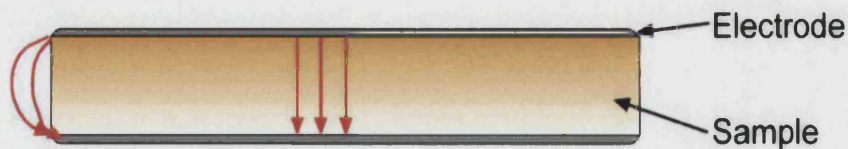
Figure 5.136: Arrows indicating non-uniform electric field at sample edge.
