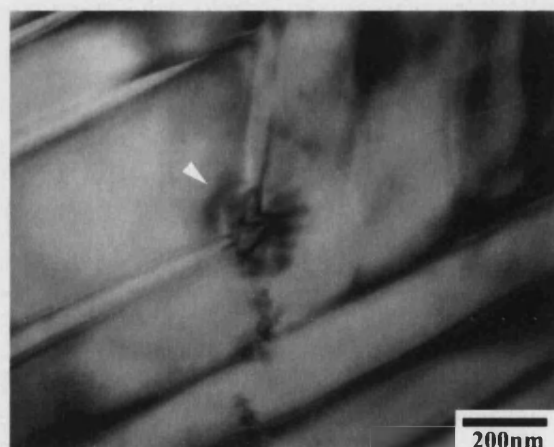
Figure 5.106: Discontinuity of domain structure at a stress concentration.
