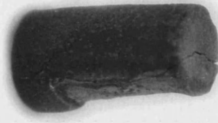
Figure 5.41: Barium titanate-5.7wt% platinum sample after dilatometry testing.
