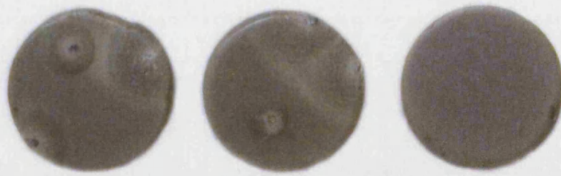
Figure 5.62: Barium titanate-1.3wt% silver showing the contact points due to additional silver loss. Sample at far right is the top surface shown for comparison.
