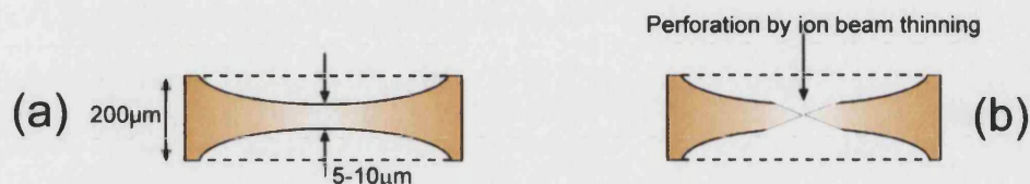
Figure AIV.9: Representation of (a) dimpled and (b) ion milled TEM specimens.
