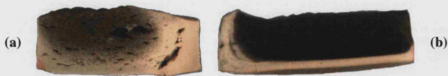
Figure 5.57: Barium titanate- (a) 2wt% and (b) 5wt% silicon carbide composites pressureless sintered at 1350°C showing chemical reduction of the barium titanate.
