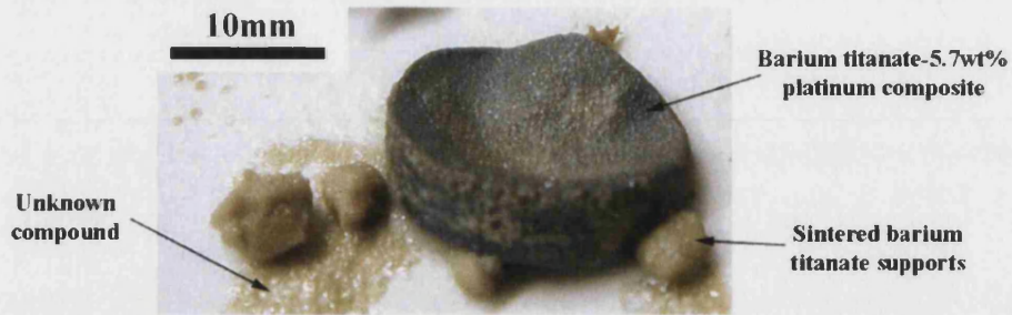
Figure 5.49: Barium titanate-5.7wt% platinum sintered at 1300°C showing amber glassy phase and differential sintering.
