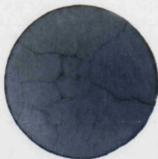
Figure 5.58: Appearance of the hot pressed monolithic barium titanate indicating a reduced state (black) and cracking. Disc diameter is 68 mm.
