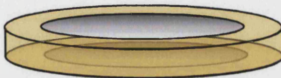
Figure 3.4: Silver electrode applied to a dielectric breakdown test sample.
