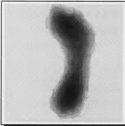
Figure 7.31 Reconstructions on the 400 element mesh using test distribution FOOT comparing the Edge and Internal electrode configurations. The element error is shown in brackets.
