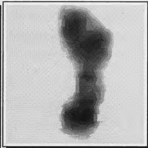
Figure 7.31 Reconstructions on the 400 element mesh using test distribution FOOT comparing the Edge and Internal electrode configurations. The element error is shown in brackets.
