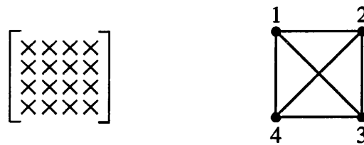
Figure A1.2 Finite element matrix and associated graph
