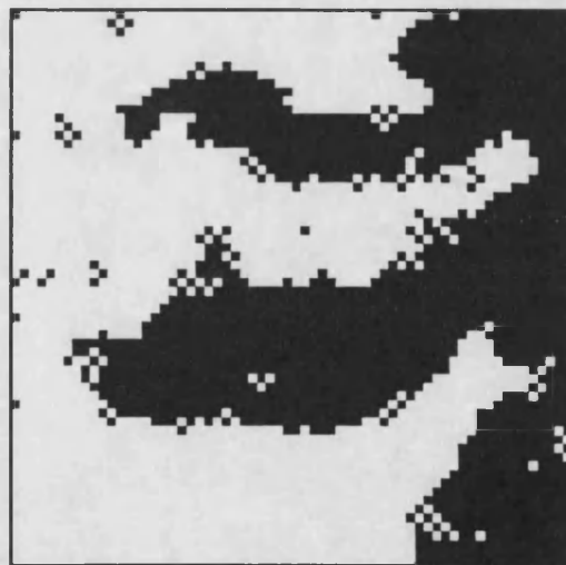
Figure 3.4 Reconstruction technique: ICM Parameters: \beta_1 = 0.0 \beta_2 = 1.0 Initial estimate: Closest mean classifier Number of pixels misclassified : 164
