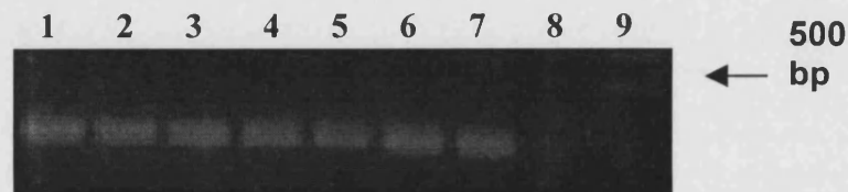
Figure 8.15 Agarose Gel showing Results of RT-PCR of E. faecium UB1 efmA Cells are Grown in Yeast Extract Medium Containing Variable Concentrations of Copper. lane 1, 10 \mu\text{M} Cu, lane 2, 5 \mu\text{M} Cu, lane 3, 1 \mu\text{M} Cu, lane 4, 0.5 \mu\text{M} Cu, lane 5, 0.1 \mu\text{M} Cu, lane 6, yeast extract supplemented with 1% foetal calf serum, lane 7, yeast extract grown cells, lane 8 no template control, lane 9, marker.
