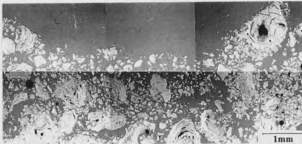
Figure 9-7 : Cross section of an indentation in IM1-24 oxidised to approximately 45% burn off, (indentation load 0.5kN).
