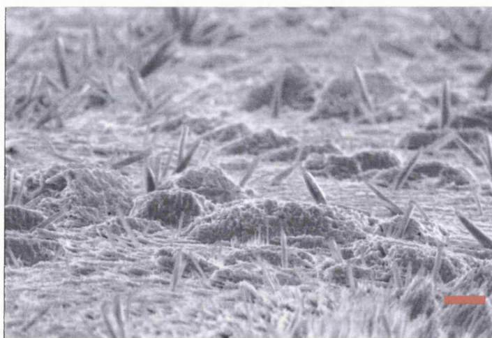
Figure 4.24 73^{\circ} tilt SEM of film grown from precursor (16) at 450\text{ }^{\circ}\text{C} on glass slides.
