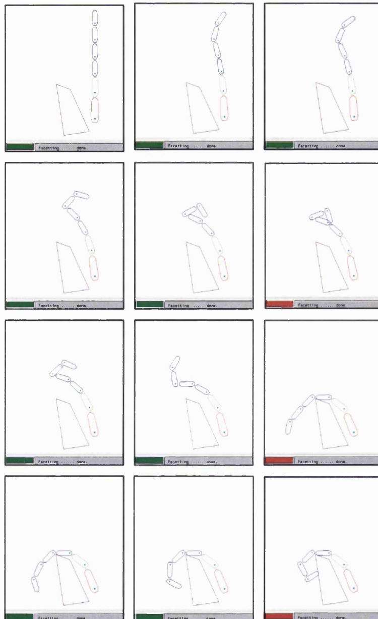
Figure 8.8: Orienter is used to explore the six-dimensional C-space map of a six-link 2-D revolute manipulator.
