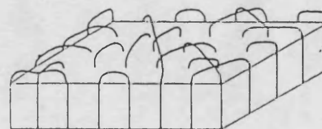
C Switchboard, or nonadjacent re-entry model in which an even more nonordered amorphous layer is present on both sides of the lamellae than in the irregular model
