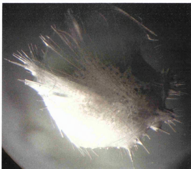
Fig 2.8c Needle crystals of LHA-S877 using hecameg detergent as additive.
