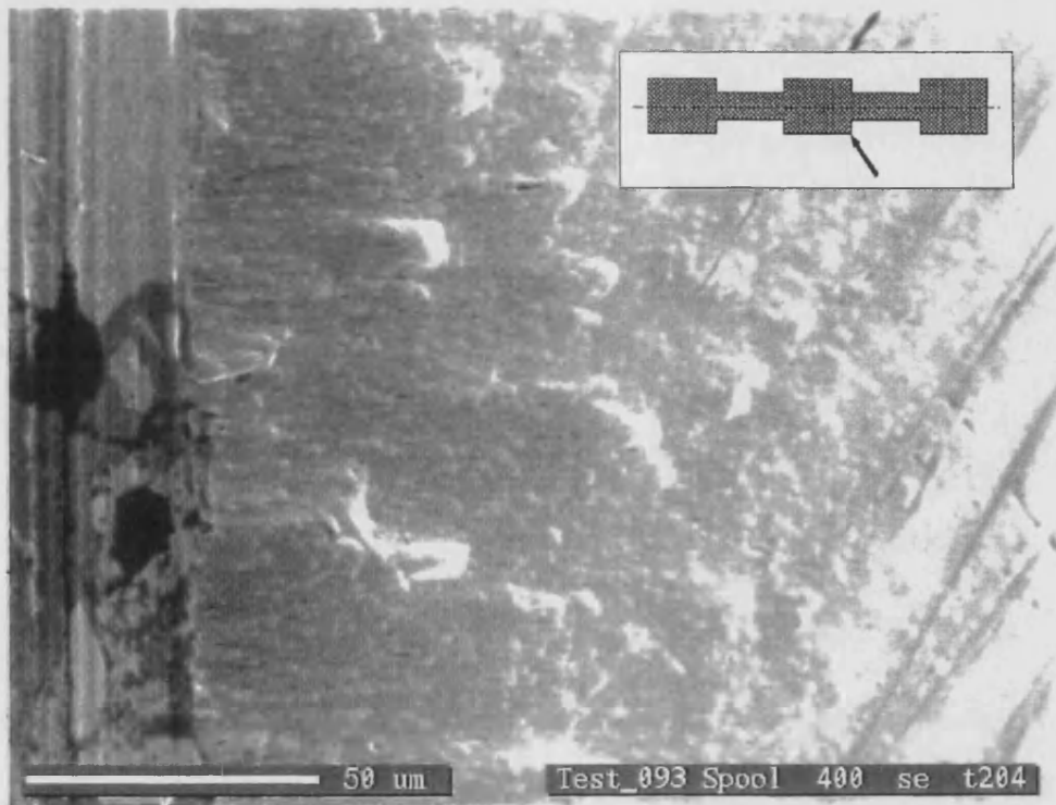
Figure 7.31 - SEM micrograph of ion implanted spool tank land, uncut quartz.
