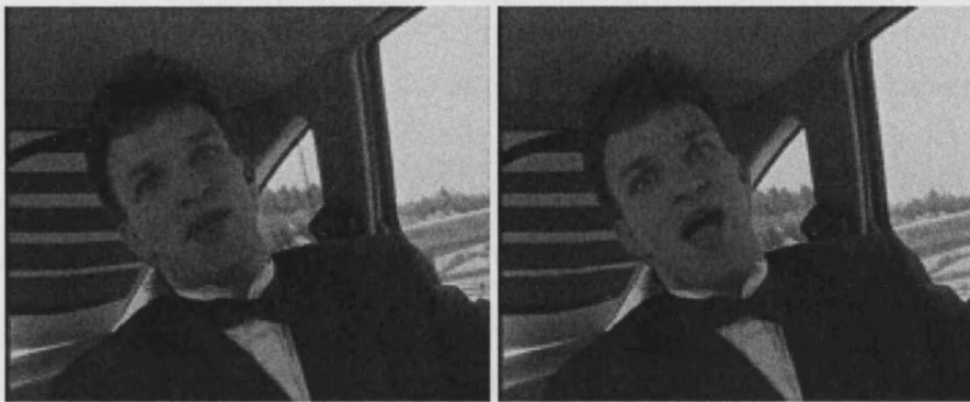
Figure 1.4: Two frames from Carphone sequence (frames 100 and 104). It is clear that there is a great deal of temporal redundancy between the frames.
