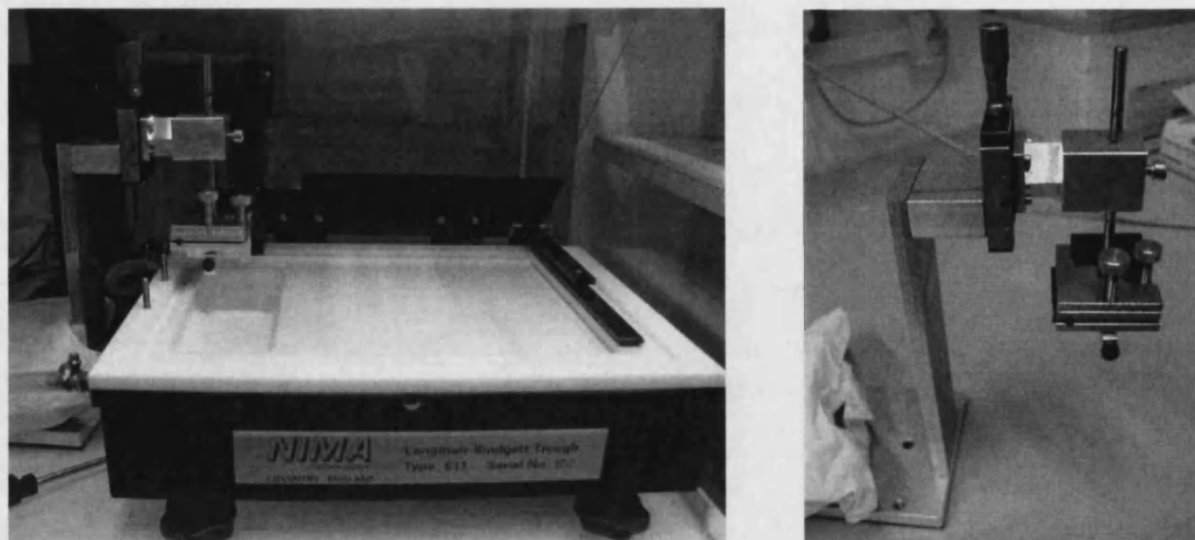
Figure 2.2 Left. Langmuir trough with dipper positioned. Right. Custom built Schaefer dipper.
