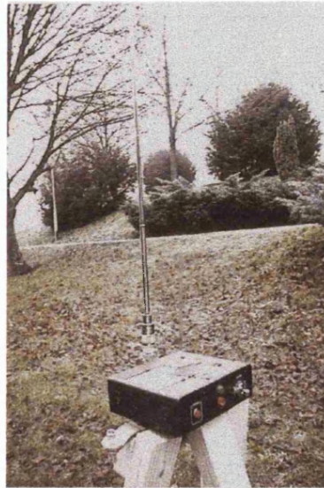
Fig. 8. 1. Wideband impulsive noise generator based on a faulty thermostat.
