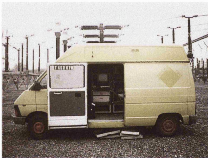
Fig. 9. 5. Equipment van for substation testing.
