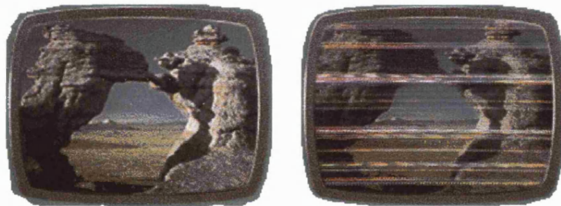
Fig. 0. 1. (a) A frame of normal TV broadcast. (b) A frame being interfered by noise generated by a faulty thermostat.
