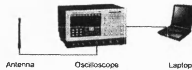
Fig. 4. The measurement configuration used for radio frequency interference measurements
