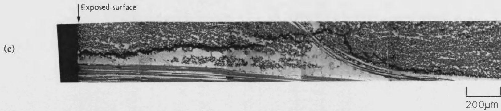
Fig.4.29 The results of DCP tests on 357-C L (2mV/min scan rate) (a) DCP curve (b) Optical micrograph taken after the test (c) Cross-section through the specimen
