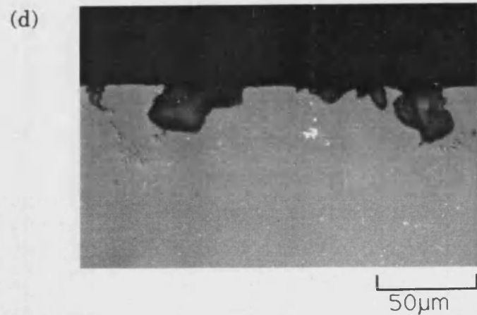
Fig.4.47 Corrosion morphology of 2124 alloy (a) After 3 days immersion, illustrating corrosion around the (\text{CuFeMn})\text{Al}_6 phase (b) After 1 week immersion (c) After 3 weeks immersion (d) Cross-section through a specimen after 3 weeks corrosion
