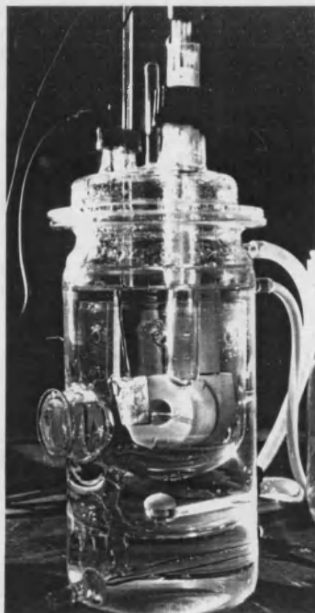
Fig.3.6 The glass cell equipped with the working, reference and auxiliary electrodes
