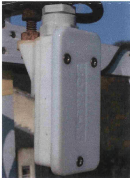
Figure 5.11: The simple vertical solar illuminance sensor supplied by the blind control manufacturer.
