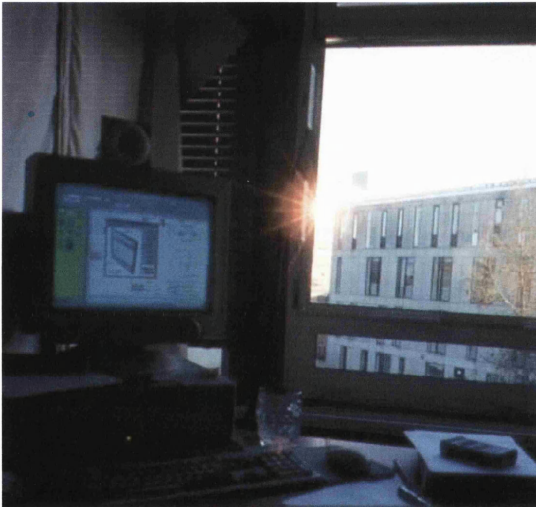
Figure 8.4: Photograph showing one of the occasions when the sun was not shining on the facade but glare reflected from an opposite building caused discomfort.
