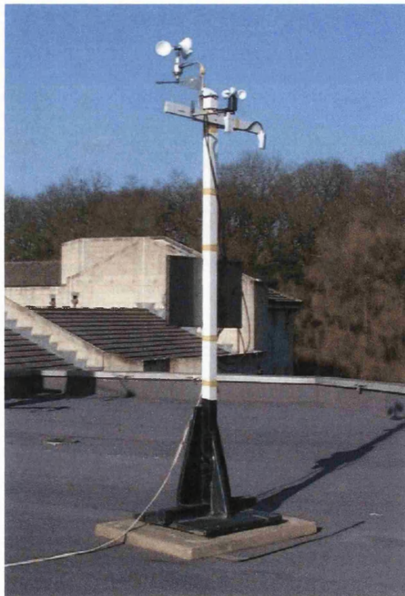
Figure 5.6: A photograph of the test room weather station located on the roof.
