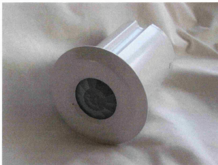
Figure 5.17: The 3 in 1 sensor with its Fresnel lens for improved occupancy sensing.
