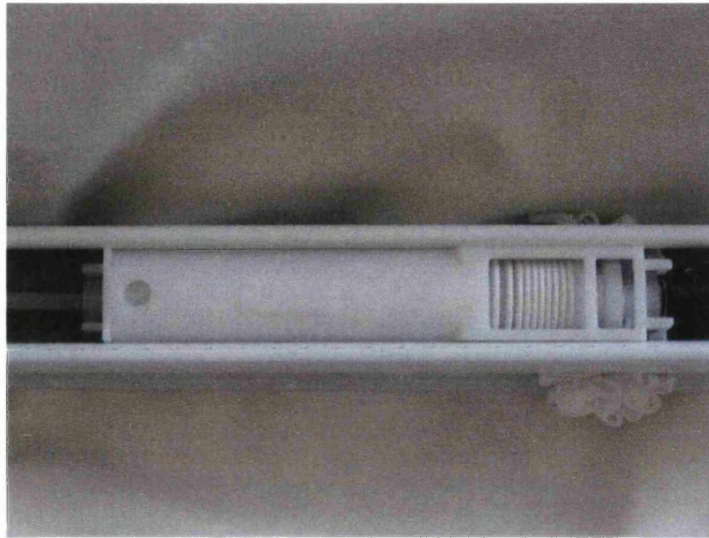
Figure 6.11: The blind head-rail cord pick-up mechanism. Through the large opening one can see the central lift cord wound around the cord collector and through the smaller opening one can see the tilt cord sitting in its groove.
