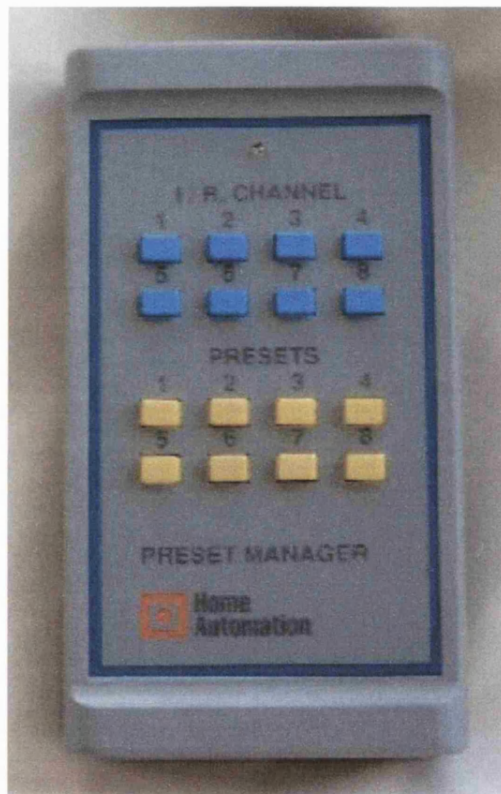
Figure 6.4: The Infra-Red Controller
