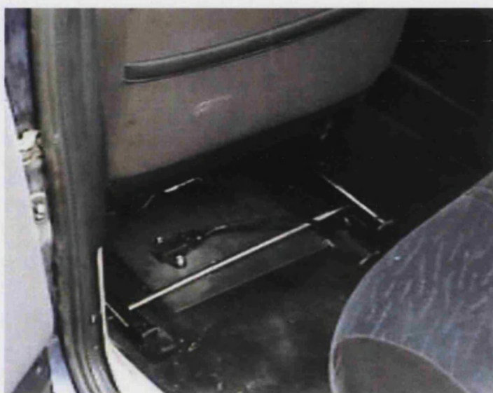
Figure 3-10 - Accelerometer mounted beneath passenger-seat
