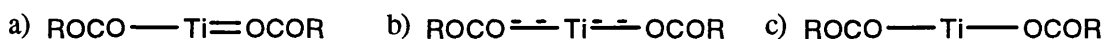
Figure 11. Suggested Ti-O bonding in titanocene bis(carboxylates). a) 18VE configuration attained though double and single Ti-O bonds. b) 18VE configuration attained though two partial Ti-O double bonds. c) 16VE configuration attained.
