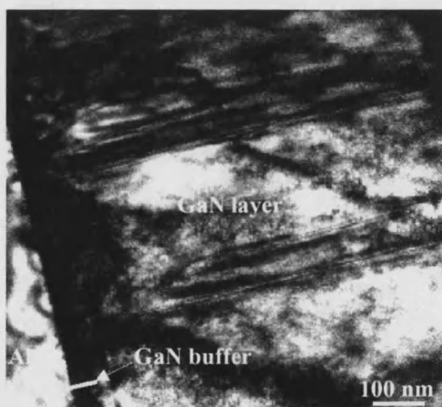
Figure 4.1 Bright field cross-sectional TEM image of the sample with (0002) reflection excited. All the defects observed in the GaN epilayer originate from those in the GaN buffer layer. (From [9])
