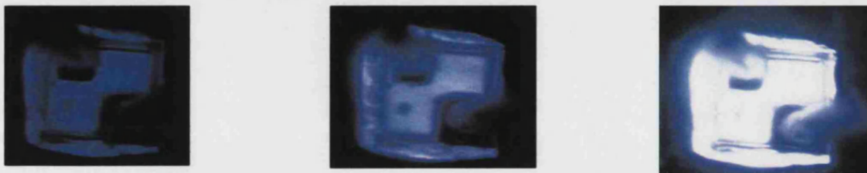
Figure 12.8 Blue light emission from LED chip at driving currents of 1 mA (left), 5 mA (middle) and 20 mA (right). Chip dimensions are 300×300 µm.
