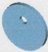
Figure 5.6: Two non-concentric circles for developing into a hollow cylindrical basic shape
