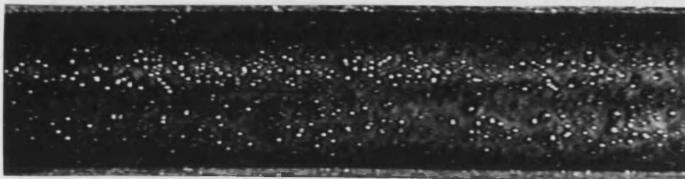
Figure 6-21 Crude Oil Fouled Test Piece
