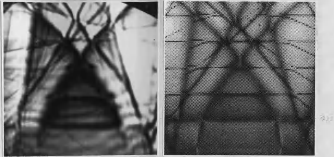
Figure 4.2.3. Experimental 200kV LACBED pattern (courtesy A G Wright) and many-beam simulation from close to Pt[231]. See text for details.
