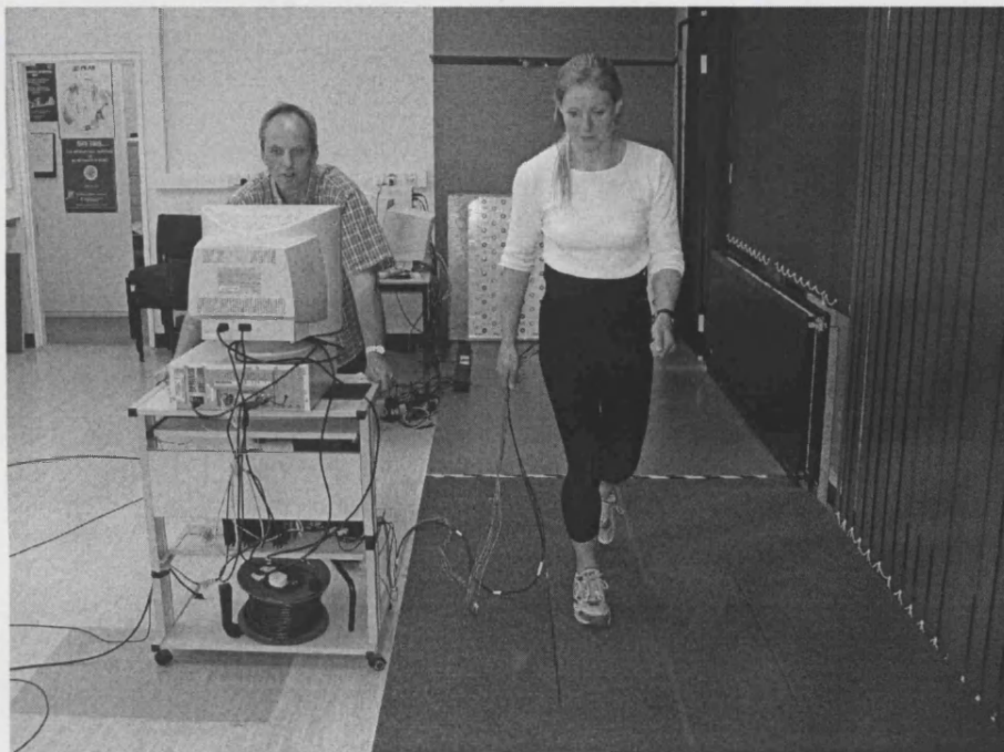
Figure B- 11 A simulation of the running experiments conducted in the Biomechanics Laboratory over the Force plate.
