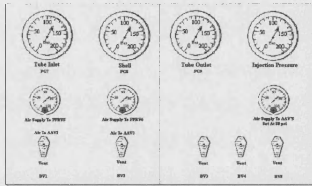
Figure 3.6: Manual Control Panel
