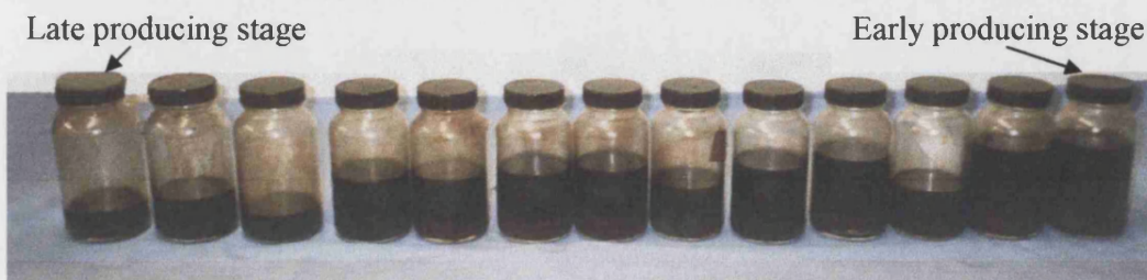
Figure 3.115: Oil and water produced from Run 1.
