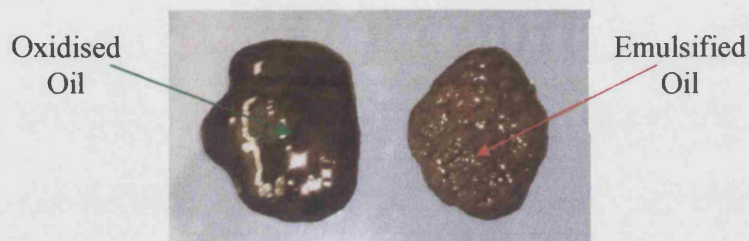
Figure 3.117: Oxidised and Emulsified Oil ( Top View )
