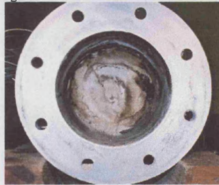
Figure 3.88 Run 2: Combustion Tube at 12 cm.
