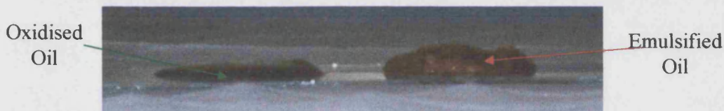
Figure 3.118: Oxidised and Emulsified Oil ( Side View )
