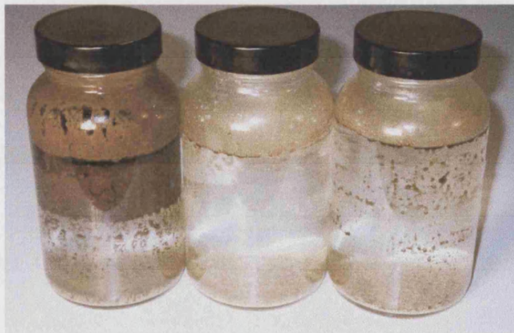
Figure 4.144: Fine Powder Deposit (Run 9).
