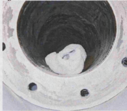
Figure 4.67 Run 4: Solid Core at 82
