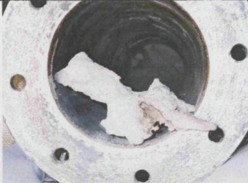
Figure 4.112 Run 8: Solid Core at 72-82 cm.
