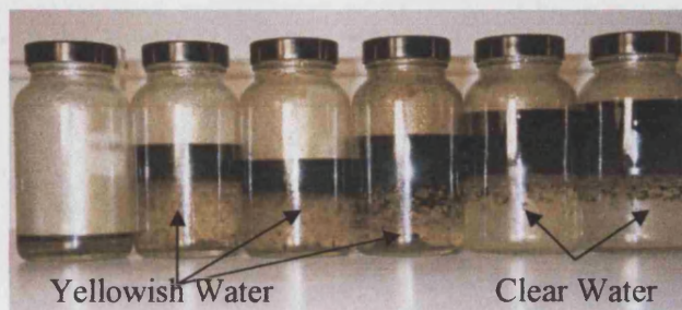
Figure 4.140: Produced Water Affected by Heat in Run 8.
