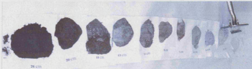
Figure 3.82 Run 1: Core samples shows extent of carbon deposition.
