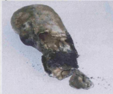
Figure 3.96 Run 2: Solid Coke at 30 – 40 cm
