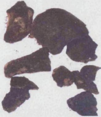
Figure 3.80 Run 1:Solid Coke at 26 cm.
