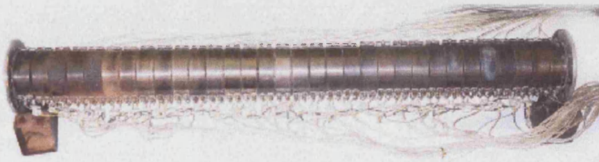
Figure 3.124: Old Sequence of Band Heaters
