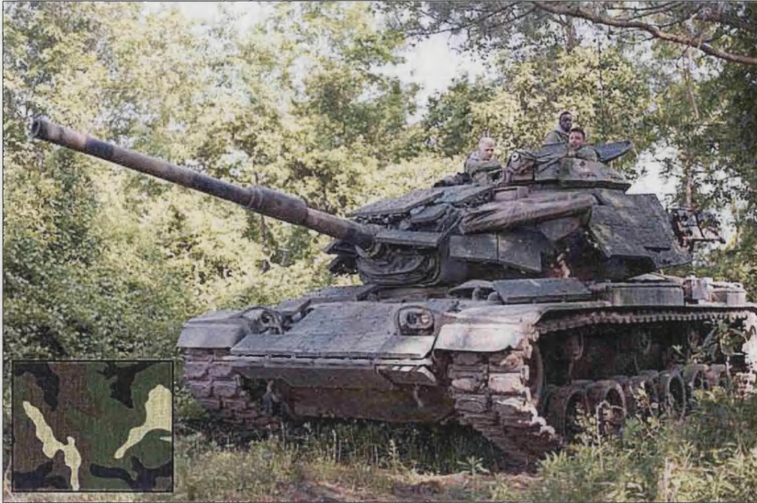
Fig. 1 An operational tank that has been painted in a disruptive pattern suitable for camouflage in a deciduous forest. The inset box shows a sample of the disruptive pattern and colours that would be used in combat uniforms for this environment.
