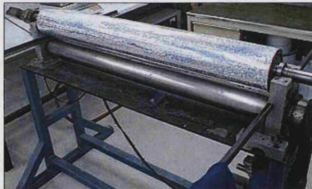
Fig. 58 A holographic metal shim is mounted on the top roller prior to embossing. Thin foil is then fed between the two rollers. This imprint is then coated in a thin protective plastic.
