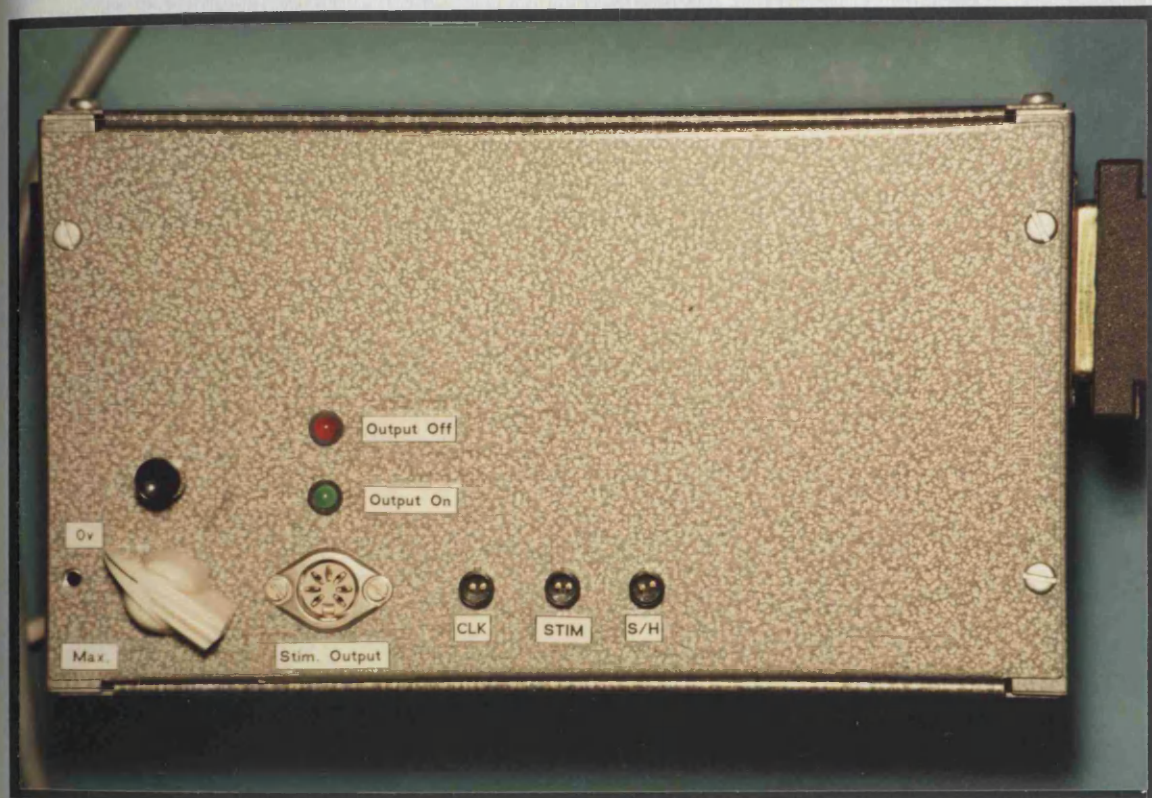
Plate F.11 Top Panel of the Power Amplifier Stimulator
