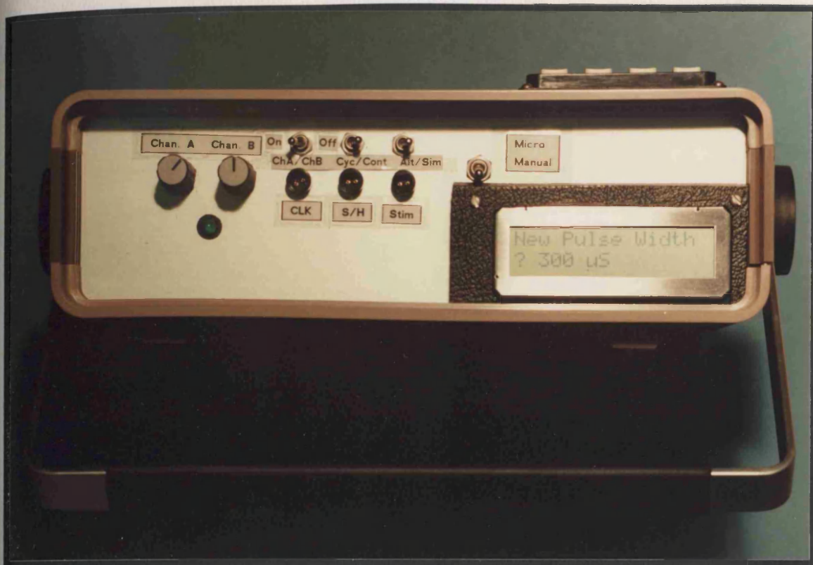
Plate F.6 Two Channel Programmable Stimulator showing the Display when Programming a New Pulse Width
