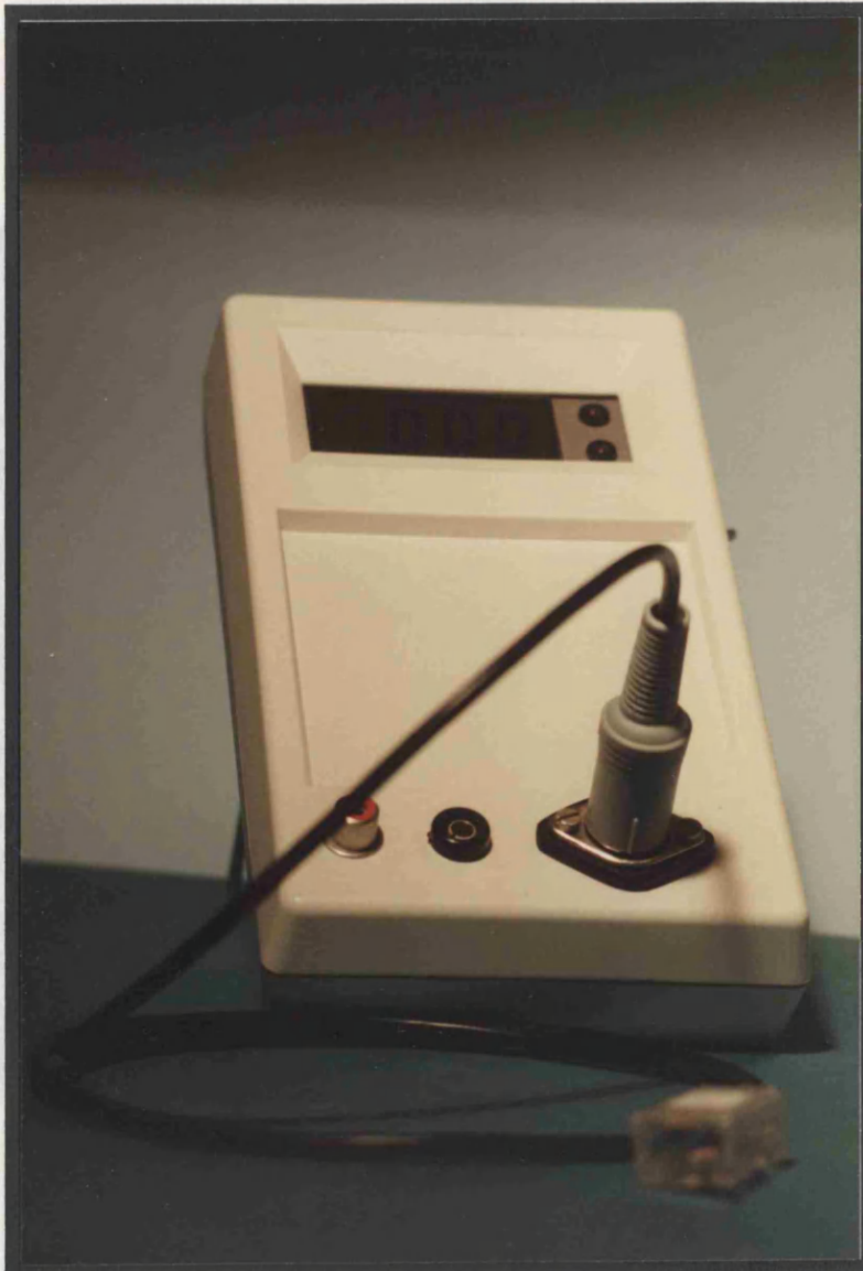
Plate F.34 Digital Muscle Fatigue Monitor Showing The Electrode Mounted Pre-Amplifier in the Foreground
