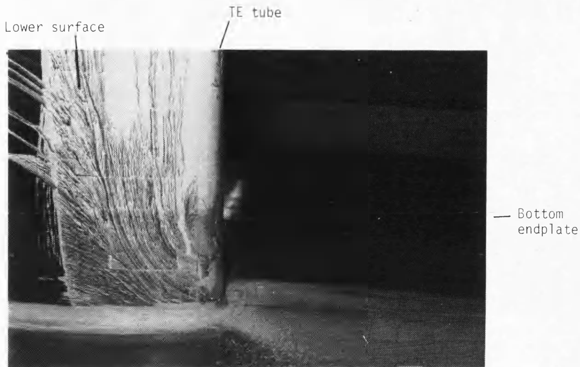
(a) Original flow near the junction between the TE tube and the bottom endplate.
