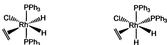
Figure 3.1. The two isomers of alkene bound intermediates, bearing trans and cis arrangements of phosphine ligands, in alkene hydrogenation by 57 .
