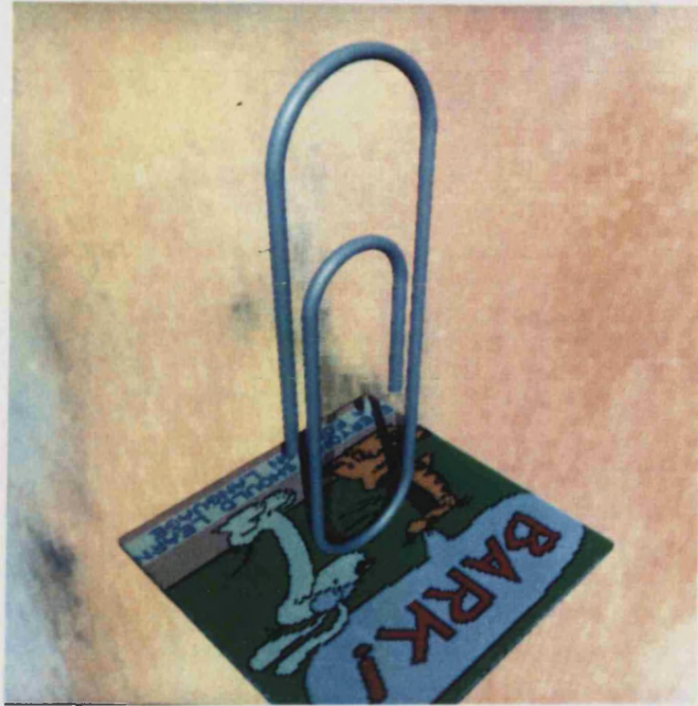
29: A CSG Model of Paper Clip Built from Cylinders, Clipping Planes and Tori
