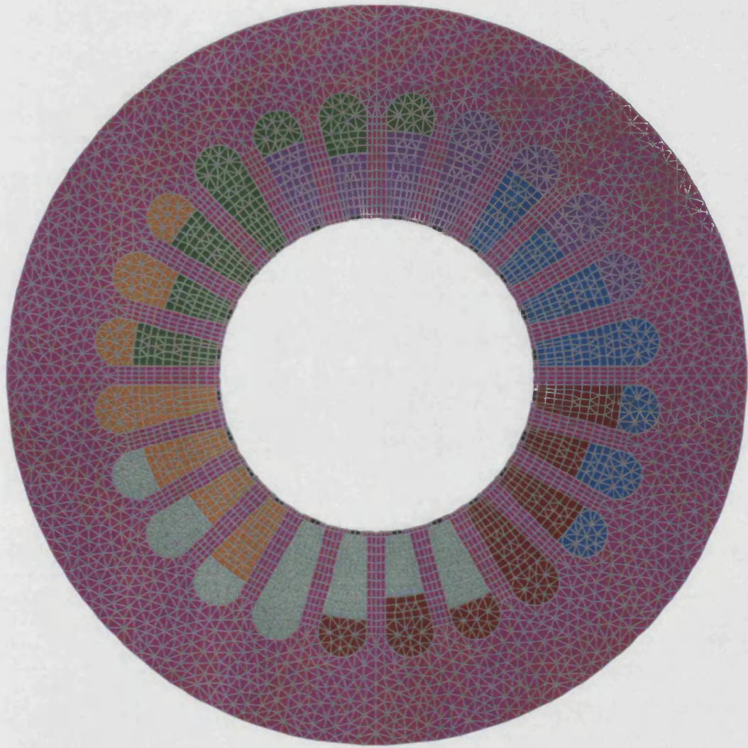
Figure 1.4: Final Stator Mesh
