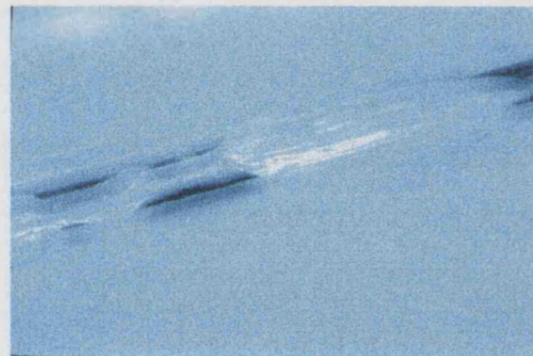
Figure 9.5 Beam 2, as the fracture front moved into the region of properly cured adhesive the failure mode became one of glass plucking.
