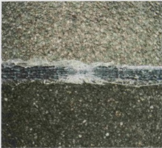
Figure 9.2 Failure origin test 1. Fracture originates from point contact with loading bar
