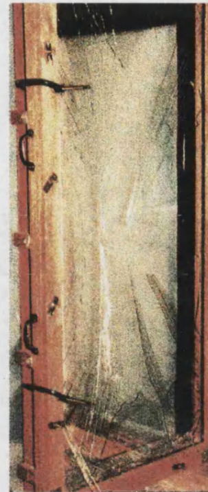
Figure 2.4 Annealed glass breaks into large dagger-like fragments
