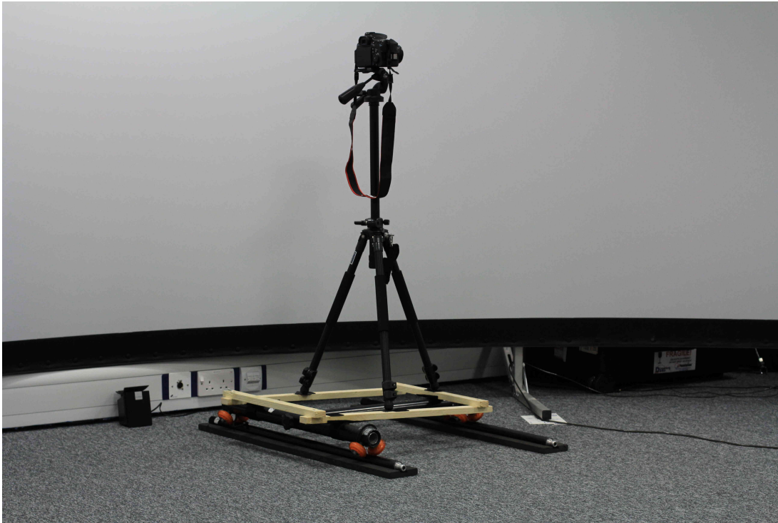
Figure 5-5: The camera rig used to take the stereo photographs.
