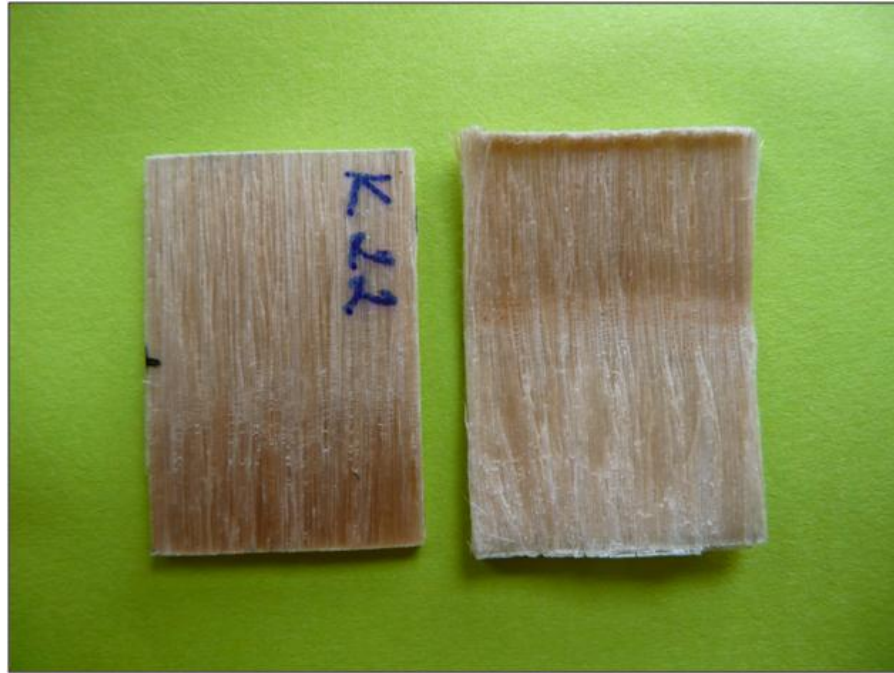
Figure 8.87: Three point bending test. Samples after fracture: compression (left) and tension (right) side of a PLA reinforced with untreated sisal fibres.
