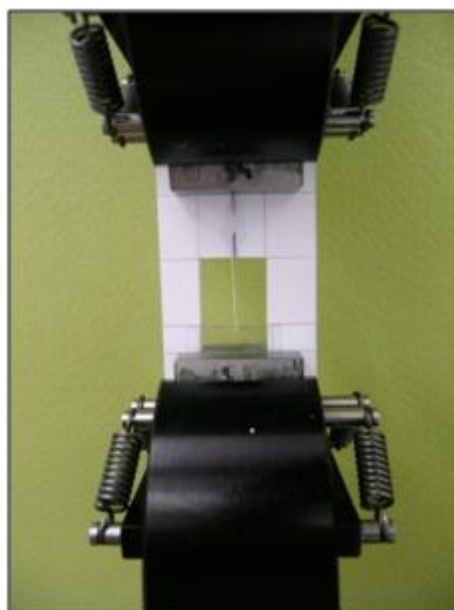
Figure 8.54: Pull-out test specimen clamped in Instron 3369 jaws prior to testing.
