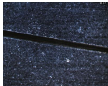
Figure A31: Non-isothermal transcrystalline growth. Caustic soda treated sisal fibre (6w%). Cooling rate 5°C/min.
