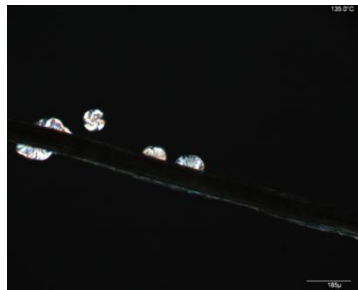
Figure A20: Isothermal spherulitic growth. Untreated sisal fibre. Cooling rate 2^{\circ}\text{C}/\text{min} . Isothermal temperature 135^{\circ}\text{C} .
