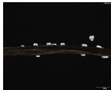
Figure A5: Isothermal spherulitic growth. Caustic soda treated sisal fibre (6wt%). Cooling rate 5°C/min. Isothermal temperature 140°C.
