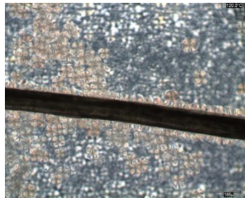
Figure A16: Isothermal transcrystalline growth. Caustic soda treated sisal fibre (2wt%). Cooling rate 5°C/min. Isothermal temperature 120°C.
