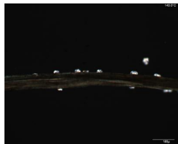
Figure A5: Isothermal spherulitic growth. Caustic soda treated sisal fibre (6wt%). Cooling rate 5°C/min. Isothermal temperature 140°C.
