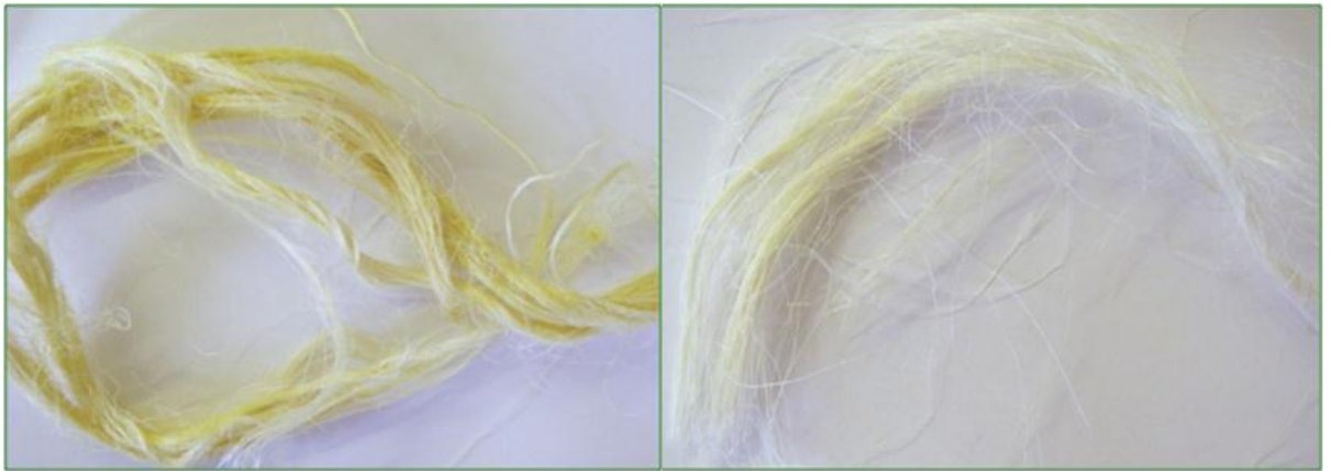
Figure 6.1: Untreated sisal fibre bundles (left) and caustic soda treated (right) sisal fibres (6 wt%).
