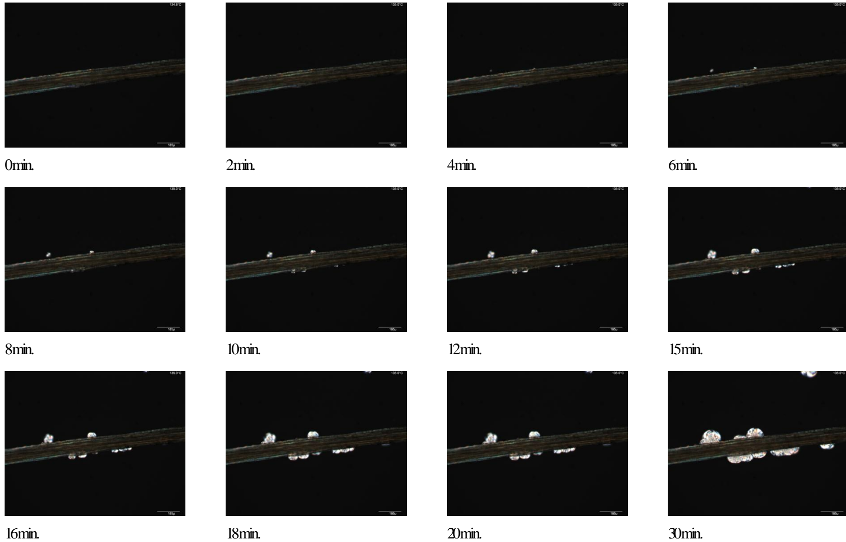
Figure A4: Isothermal spherulitic growth. Caustic soda treated sisal fibre (6 wt%). Cooling rate 5°C/min. Isothermal temperature 135°C.
