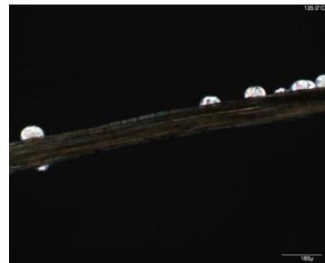
Figure A9: Isothermal spherulitic growth. Caustic soda treated sisal fibre (6wt%). Cooling rate 2°C/min. Isothermal temperature 135°C.
