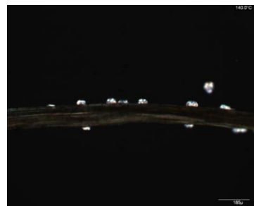
Figure A5: Isothermal spherulitic growth. Caustic soda treated sisal fibre (6wt%). Cooling rate 5°C/min. Isothermal temperature 140°C.
