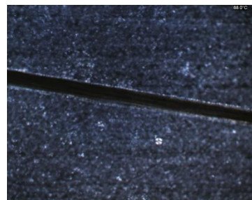
Figure A31: Non-isothermal transcrystalline growth. Caustic soda treated sisal fibre (6w%). Cooling rate 5°C/min.
