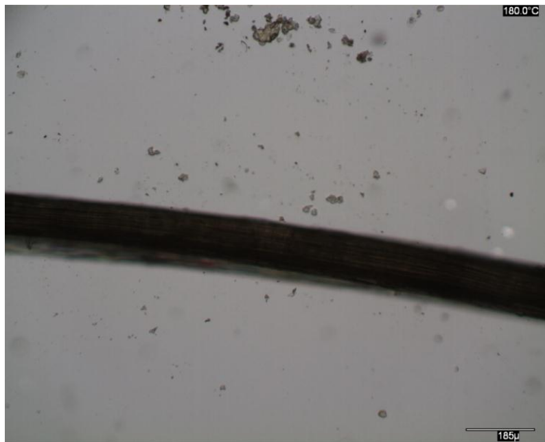
Figure 8.46: Microcrystalline cellulose washed out from the caustic soda treated sisal fibre.
