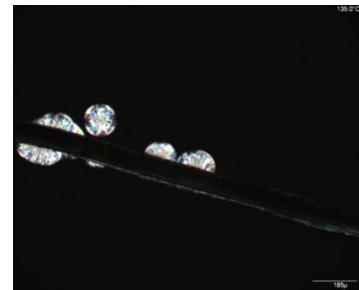
Figure A20: Isothermal spherulitic growth. Untreated sisal fibre. Cooling rate 2^{\circ}\text{C}/\text{min} . Isothermal temperature 135^{\circ}\text{C} .
