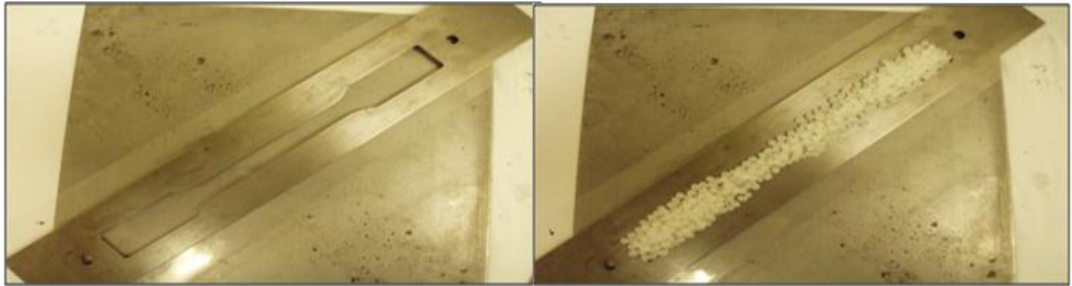
Figure 7.1: Compression mould for PLA dog bone samples for tensile testing. Open mould (left) and the mould filled in with PLA granules.
