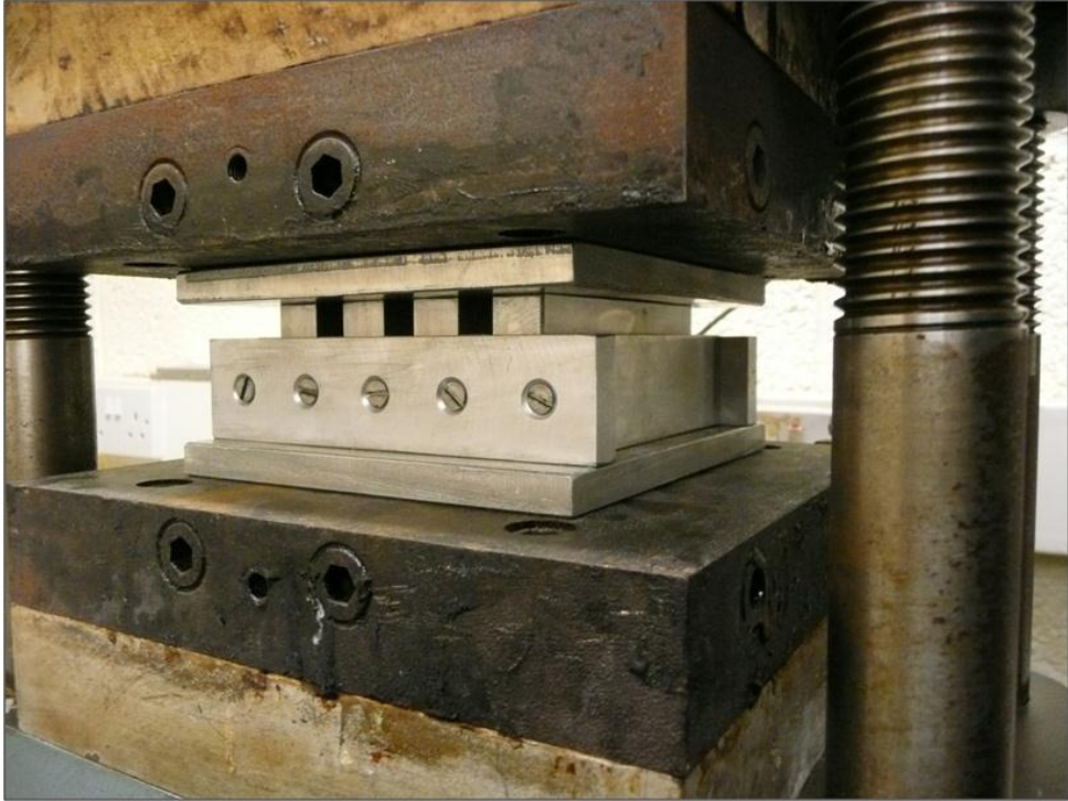
Figure 7.18: Mould transferred into a hot press.
