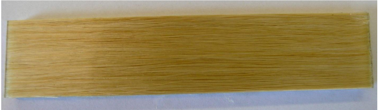
Figure 7.19: PLA / sisal fibre unidirectional composite (100 x 15 x 1 mm).
