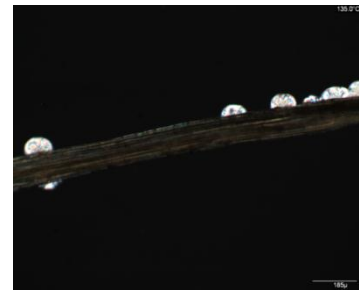
Figure A9: Isothermal spherulitic growth. Caustic soda treated sisal fibre (6wt%). Cooling rate 2°C/min. Isothermal temperature 135°C.
