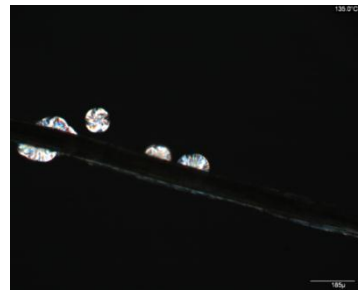
Figure A20: Isothermal spherulitic growth. Untreated sisal fibre. Cooling rate 2^{\circ}\text{C}/\text{min} . Isothermal temperature 135^{\circ}\text{C} .
