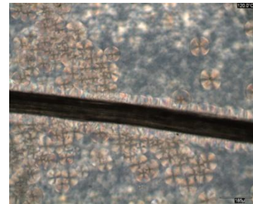
Figure A16: Isothermal transcrystalline growth. Caustic soda treated sisal fibre (2wt%). Cooling rate 5°C/min. Isothermal temperature 120°C.
