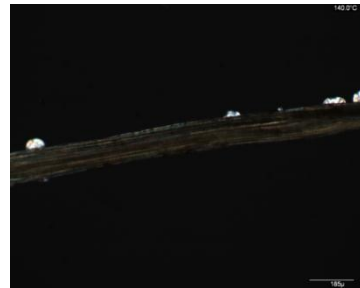
Figure A10: Isothermal spherulitic growth. Caustic soda treated sisal fibre (6wt%). Cooling rate 2°C/min. Isothermal temperature 140°C.
