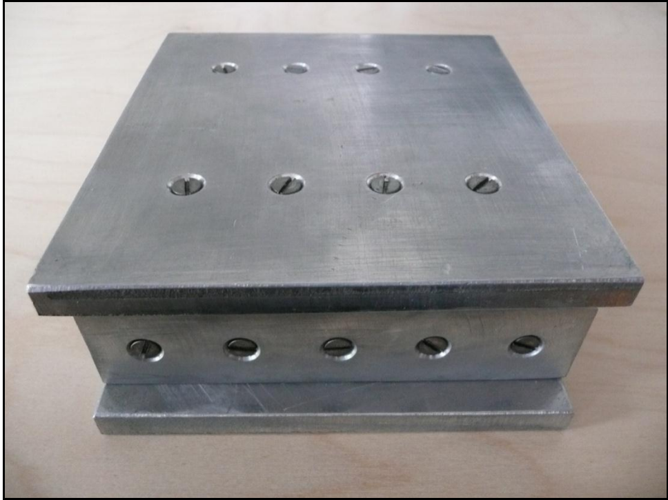
Figure 7.17: Closed mould prepared for hot pressing.
