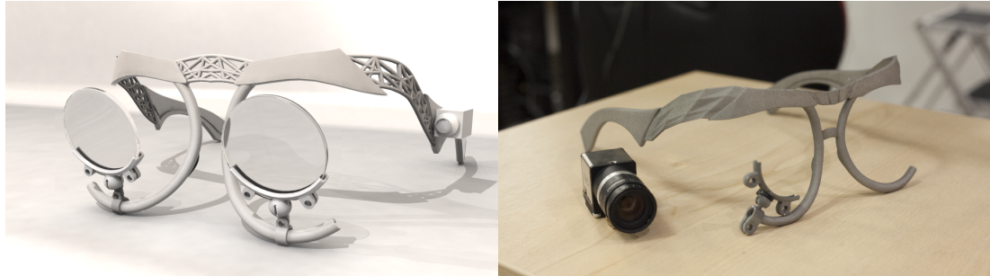
Figure 5-10: Virtual model (left) and physical model (right) of our prototype head-mounted eye tracking frame, developed with help from resident Disney artists. Pictured also is an IDS UI-3370CP NIR machine vision camera, which is the model being used for our solution. It is equipped with a 12mm FL lens.
