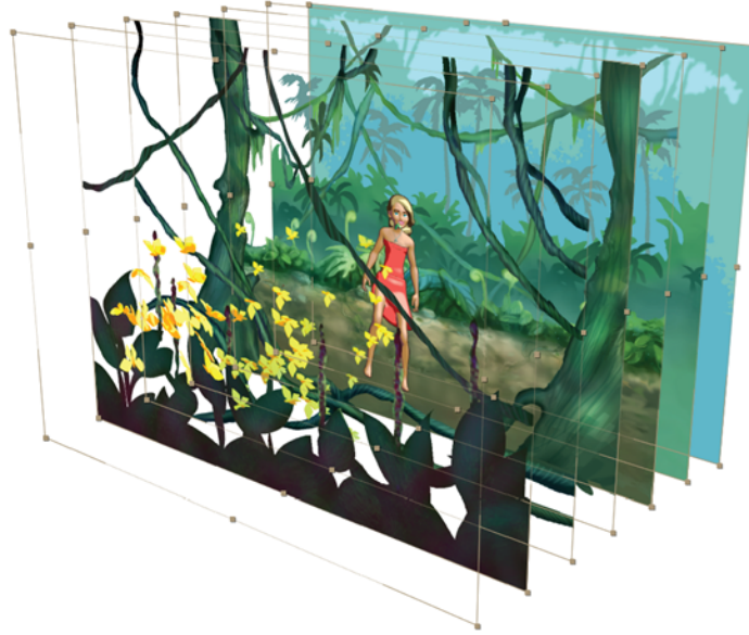
Figure 5-3: The layered 3D video format. Each layer can be animated in order to present dynamic content. The illusion of depth is provided via parallax, with layer distances specified in the video container.
