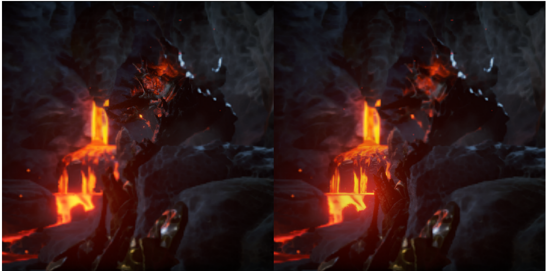
Figure 4-2: Comparison stills of the foveated rendering implementation within Unreal Engine 4 on the Elemental Tech Demo provided by Epic Games, Inc. The peripheral layer is upscaled from a lower resolution render and the foveal layer rendered at native density. On the left, the foveal region is focused on the character. On the right, the foveal region is focused on the lava fall behind him.
