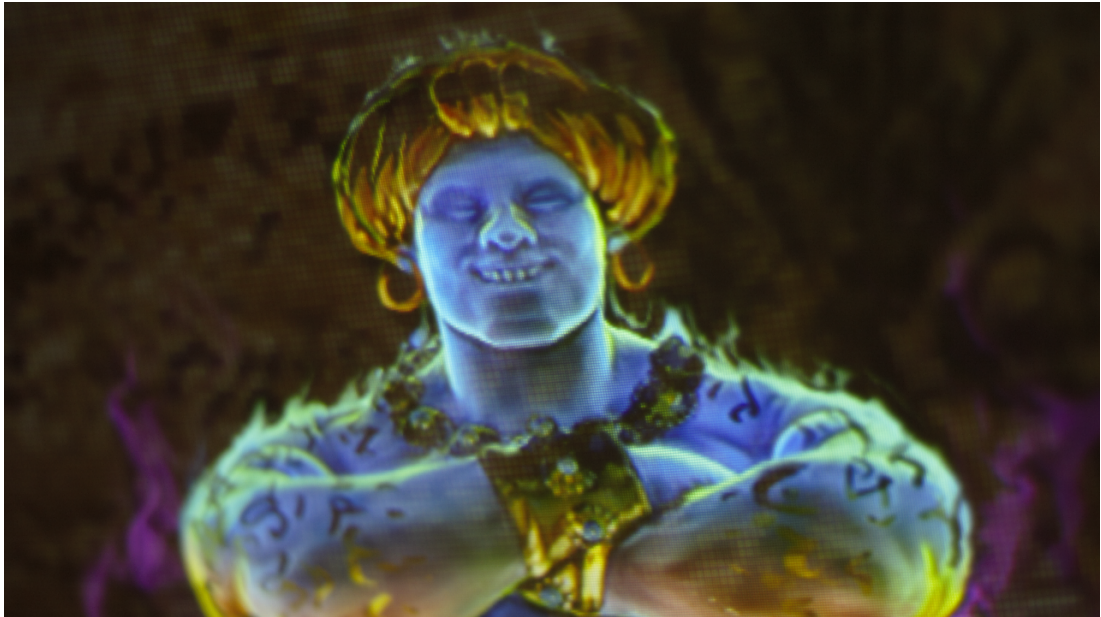
Figure 5-7: Close up view of the quality difference between projections. The foveal projector, displaying the genie, operates at a much higher pixel density than the peripheral projection, displaying the desert background. Although visible blending and transparency issues and transparency could be somewhat alleviated by a mask in the peripheral projection, there will always be a need for blending on window edges as the content refresh rate of the projector (60 Hz) cannot match the speed of the motors and may cause visible artifacts after a saccade.
