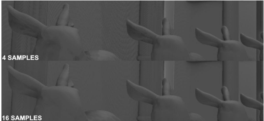
Figure 4-4: Strips from two foveated renders with the same fixation point but different peripheral sampling levels. Fixation point is at the bottom-right corner for each strip. Transition between foveal and peripheral regions are handled smoothly. At 4 samples there are noticeable artefacts, such as banding on the wall.
