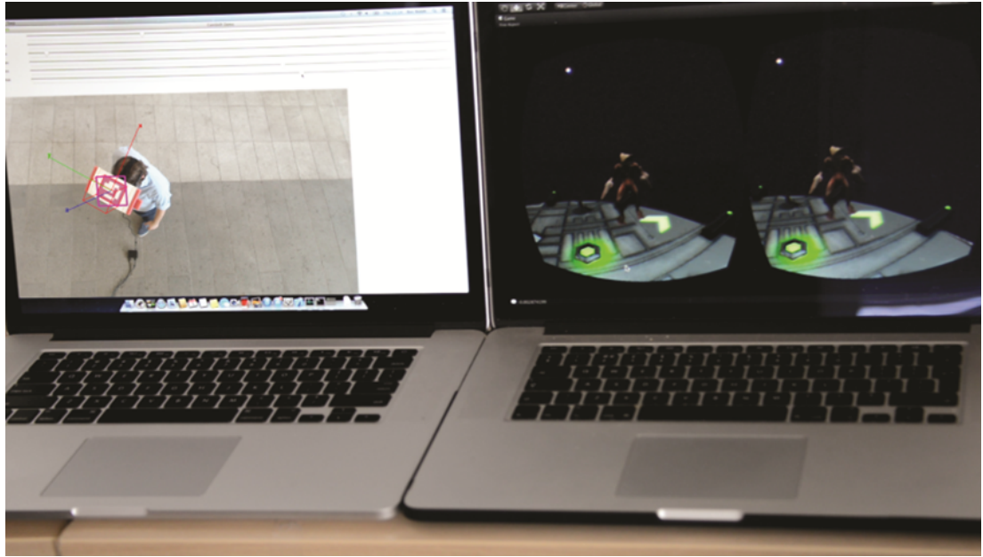
Figure 5-2: Our system running across multiple machines. The laptop on the left (server) conducts the image-based tracking. The position and orientation data is wirelessly transmitted to the laptop on the right (client). This data is then Kalman filtered against the HMD’s tracking data, which is connected to the client machine.
