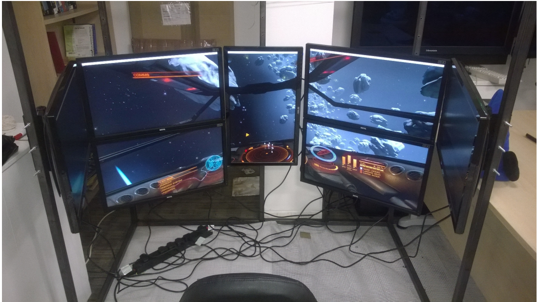
Figure 5-4: Image of the prototype multi-monitor VRE. The system used three Asus VG278HE 27” monitors (central portrait and far edges) and four BenQ XL2720Z 27” monitors (flanking the central portrait monitor). The system is running Elite Dangerous at 8760x2160 resolution.
