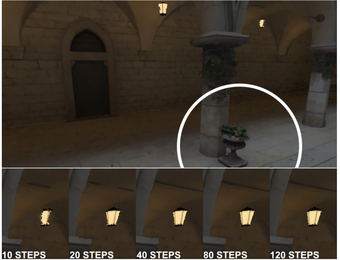
Figure 4-6: Top: Sample frame from our ray-casting method with 120 per-pixel steps in the foveal region (within circle) and 10 per-pixel steps in the peripheral region (outwith circle). Bottom: Close-up of right lamp showing artefacts across different quality levels.
