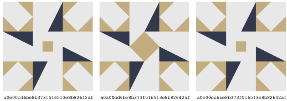
Figure 2.1: Visualising hash keys for easy comparison : In the examples shown, an original Md5 hashed key is compared with two others (one identical, one not). By modulating the raw key to an image, identifying the odd-one-out is made much easier for the human perceptual system to detect.
