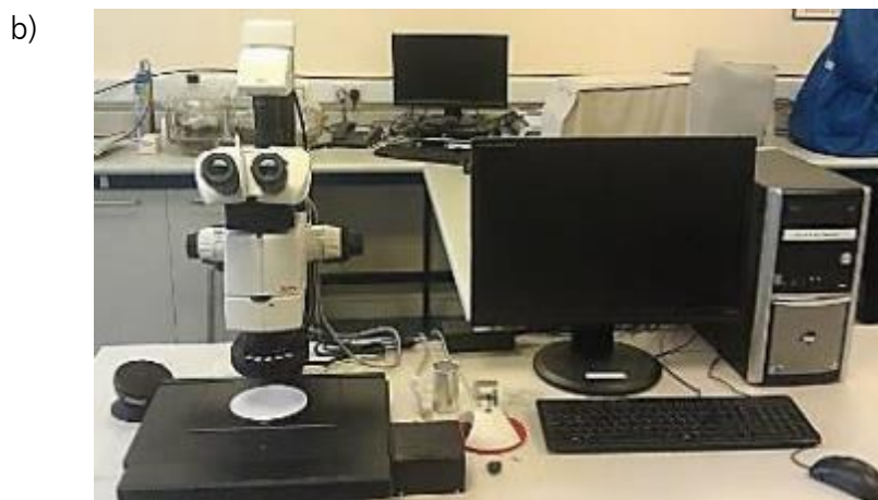
Figure 6-11. a) Leica DM ILM inverted microscope. b) Leica M 205C stereomicroscope.
