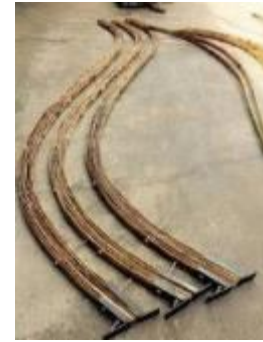
Figure 11-13. Bamboo bent for the roof structure of a tent ( http://www.giantgrassdesign.com )
