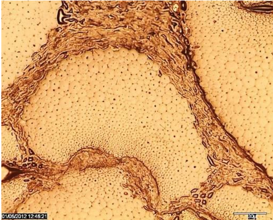
Figure 6-15. Inverted microscope image of a vascular bundle following densification (sample C). Taken with a Leica DM ILM at 10x magnification.
