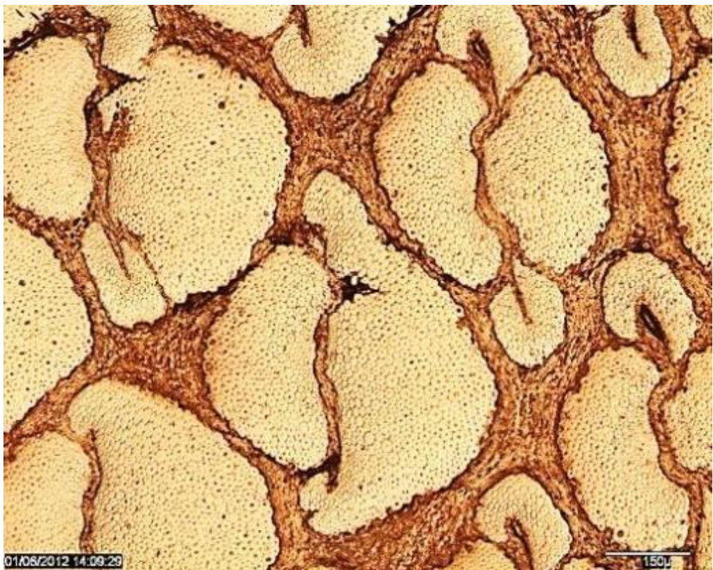
Figure 6-14. Inverted microscope images of a specimen of sample C at 10x magnification. a) Vascular bundles with surrounding parenchyma cells and conductive after densification of a specimen close to the cortex. b) Vascular bundle following densification of a specimen from the middle part of the culm.
