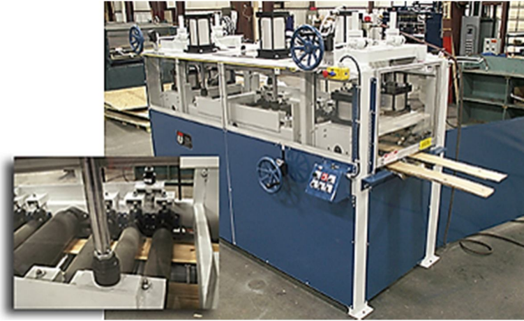
Figure 11-5. Multi-nip rotary laminator for engineered flooring with hot melt roller coaters ( http://www.uniontoolcorp.com ) whose design could be adopted for continuous densification of Guadua strips.
