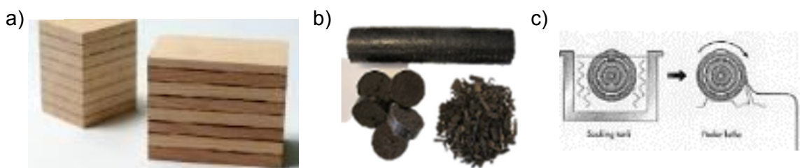
Figure 4-8. THM wood modifications. a) Layers of beech and spruce bonded by circular friction welding ( www.ibois.epfl.ch ). b) Torrefied wood briquettes ( www.cfnielsen.com ). c) Wood veneer processing by steaming and boiling of logs prior to peeling ( www.madehow.com ).
