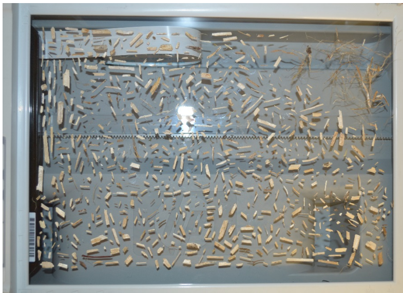
Figure 4.2: Segregated aggregate particles prior to scanning for two dimensional image analysis.
