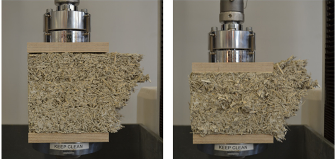
Figure 4.17: Compressive testing of a non-resized flexural specimen half.
