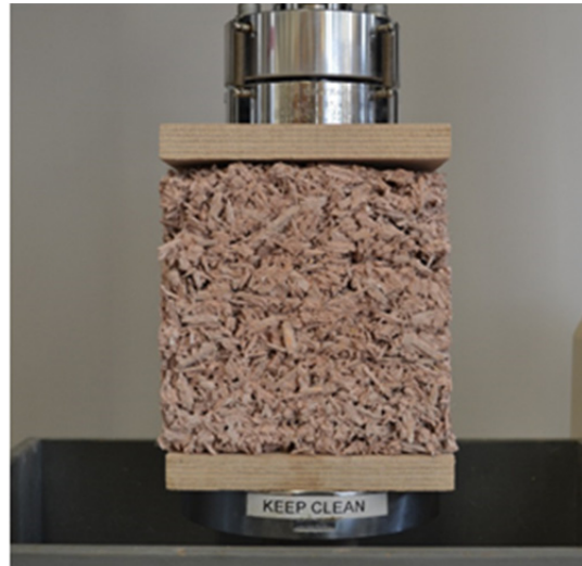
Figure 4.15: Diagrammatic and actual testing of hemp-lime in compression.
