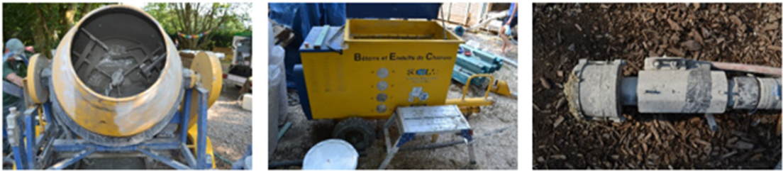
Figure 4.21: The three parts of the projection forming equipment. Left to right: the slurry mixer/agitator and pump, the aggregate hopper and air blower, the application lance.
