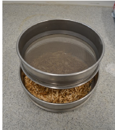
Figure 4.5: Sieves used to measure water absorption of aggregates.
