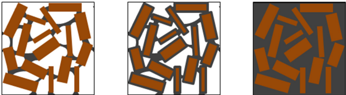
Figure 2.6: Diagrammatic representation of the three phases of structure at differing binder concentrations as proposed by Cerezo (Cerezo, 2005).
