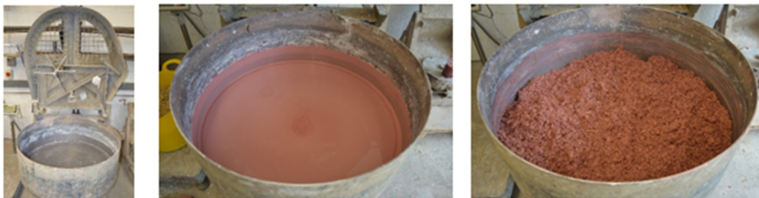
Figure 4.19: The mixing process. Left to right: the pan mixer, the slaked binder with pigment dose added, the final combined mixture.
