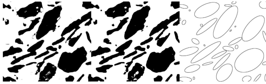
Fig. 4. Left to right: thresholded image, image passed through opening algorithm, image assessed for particles and represented as best fitting ellipses.
