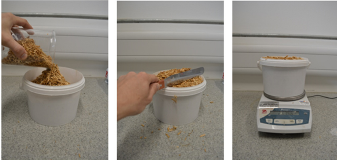
Figure 4.4: The process of determining bulk density of loose hemp-shiv.
