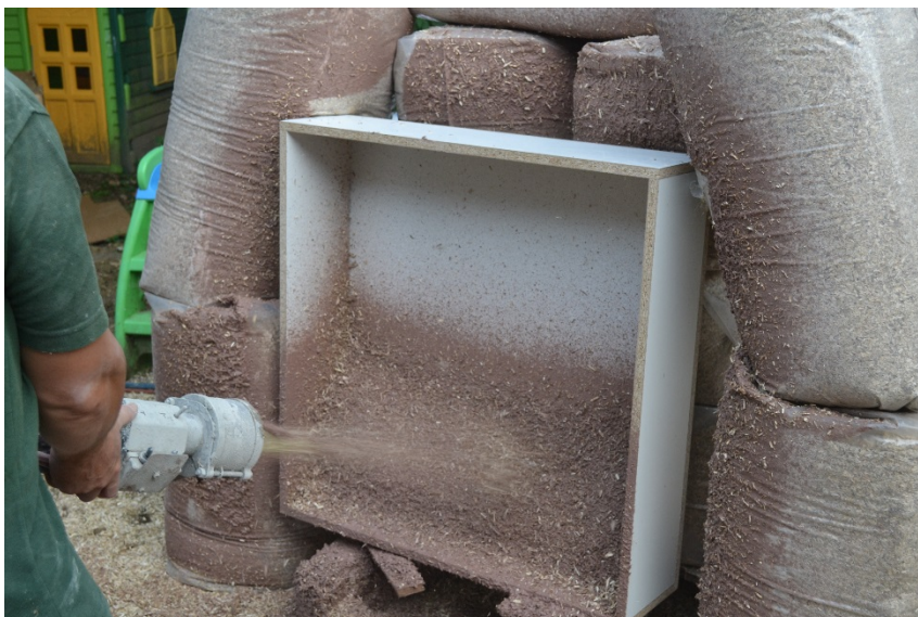
Figure 4.22: The production of the projection formed specimens by Hemp-lime Spray.
