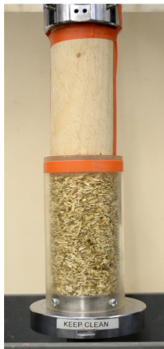
Figure 4.8: The loose hemp load cell installed within the Instron 50KN frame.
