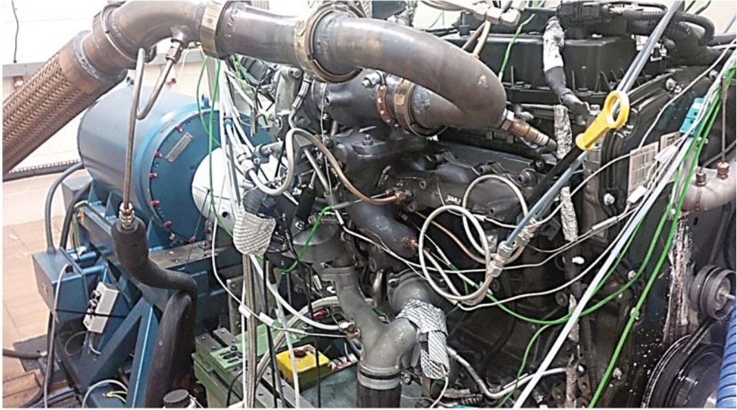
Figure 7.7 the fully instrumented two stage system installed on the baseline engine
