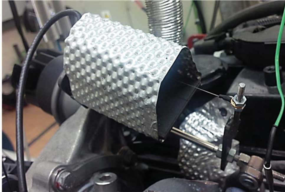
Figure 7.3 pull wire valve travel sensor and the heat shield
