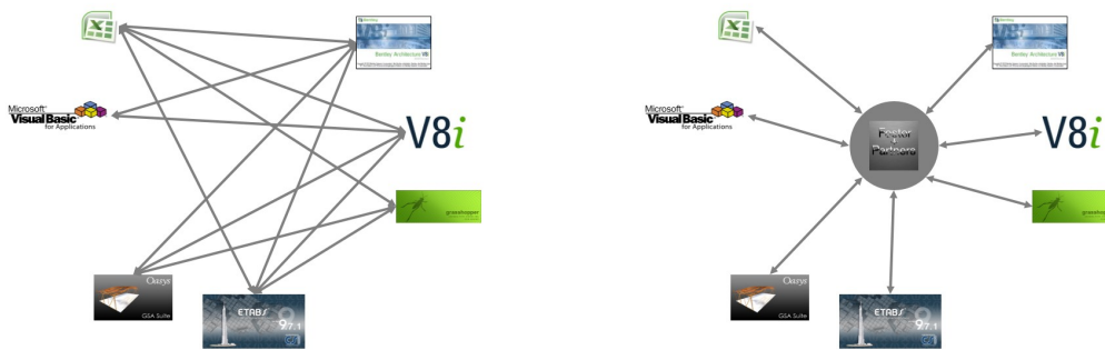
Figure 2-12: Example showing the number of links required to link programs if implemented as a one-to-one set of links or to a central hub. Source Author
