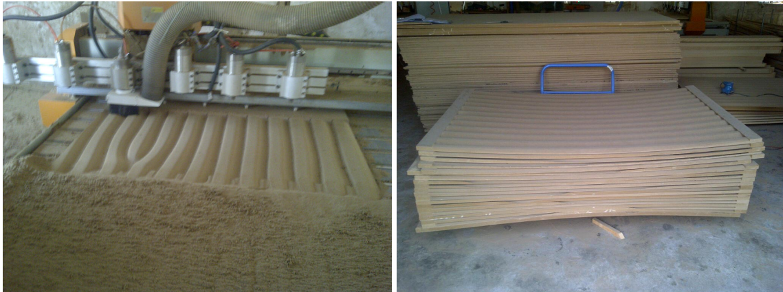
Figure 4-6: CNC Machine cutting UAE Pavilion's sand ripple mould liners. Source Foster + Partners.
