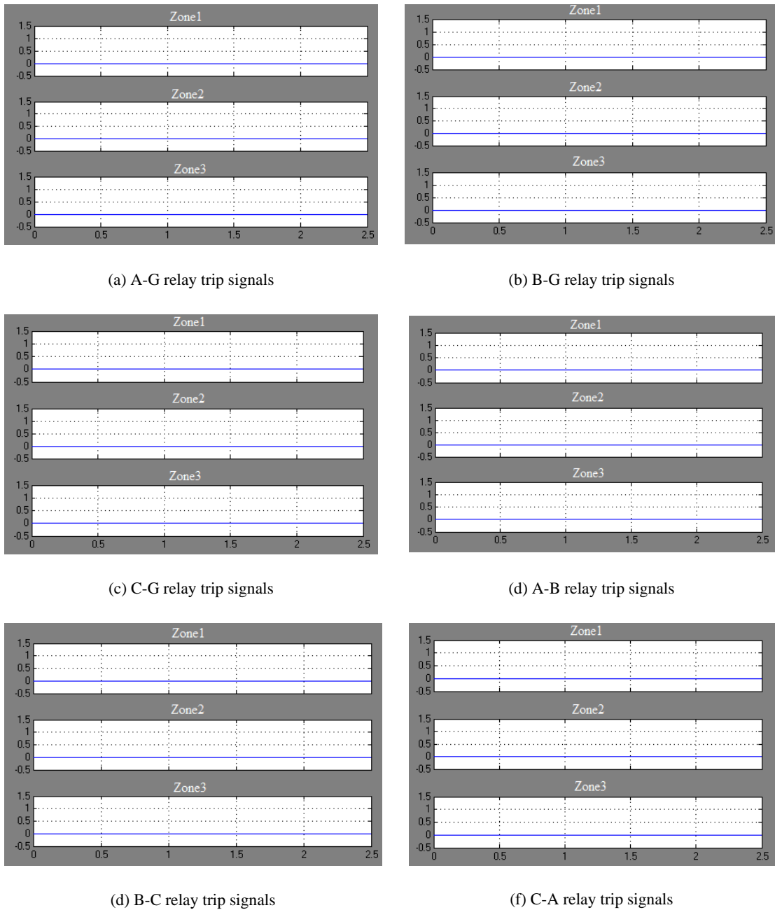
Figure 7-27 Distance relay trip signals for an A-G fault on the HVAC line beyond the DC link in the HVAC/HVDC transmission system
