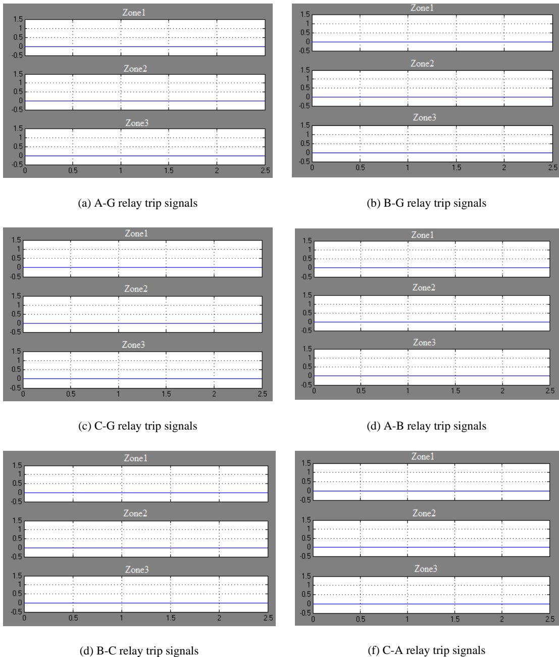
Figure 7-14 Distance relay trip signals for a zone2 fault in the HVAC/HVDC transmission system
