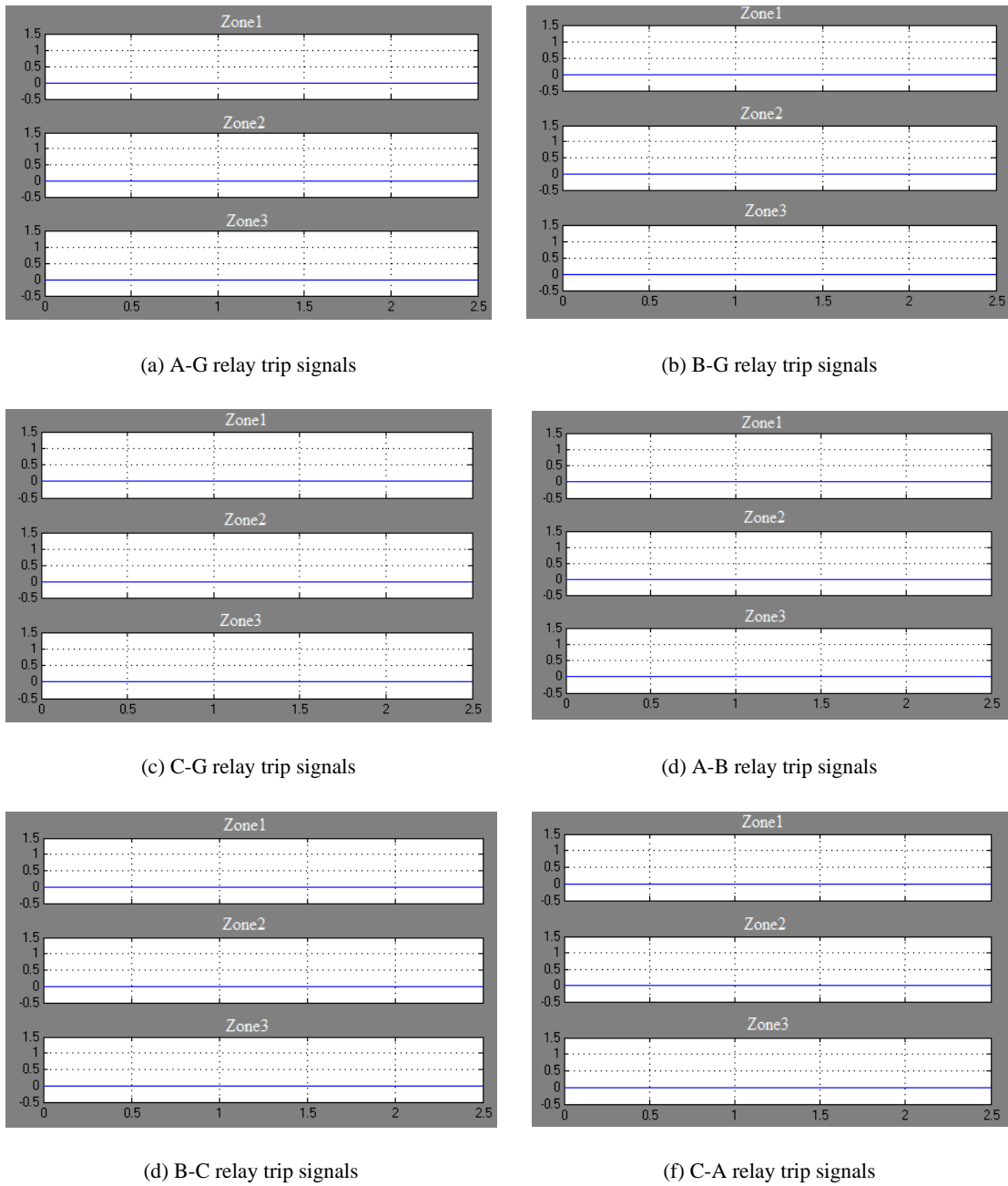
Figure 7-31 Distance relay trip signals for fault at 200km from the relay point on the HVAC/HVDC transmission system
