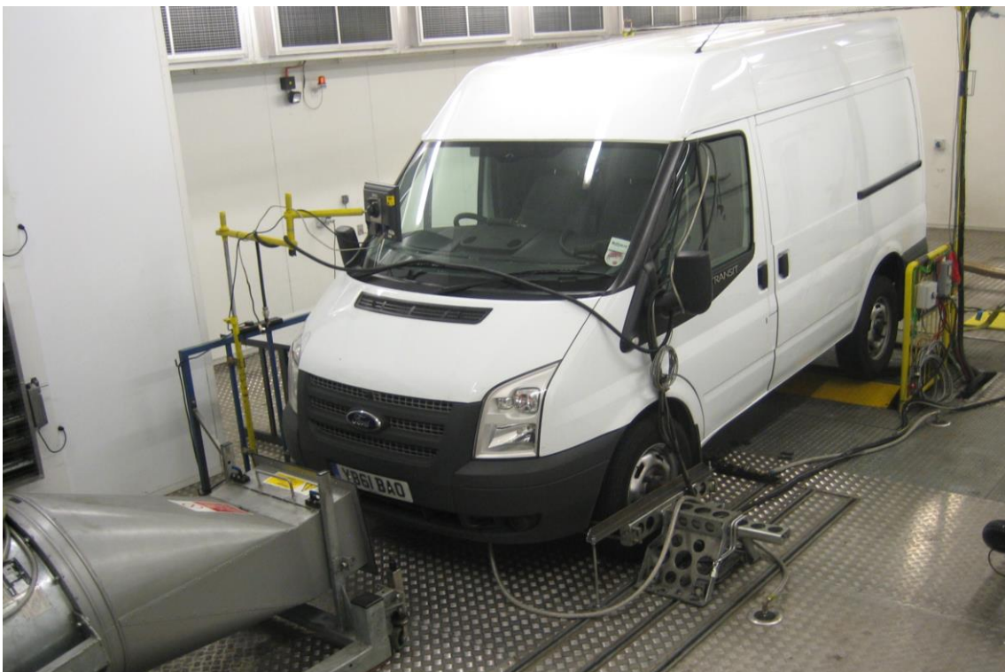
Figure 6-5: Vehicle installation on the chassis dynamometer test facility. Road speed fan can be seen in the bottom left of the photo, and the driver's aid display in front of the windscreen.
