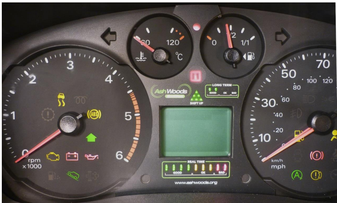
Figure 3-2: Photograph showing a vehicle instrument cluster with Lightfoot during key-on initialisation. The Lightfoot add-on can be seen in the centre; LEDs indicating IPS_{ST} are below the standard vehicle computer screen, and those indicating IPS_{LT} and the GSI are positioned above the screen.
