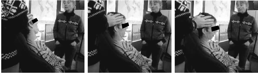
Figure 12-8: A series of three photographs of Daniel during his evaluation of a soft prototype of a dynamic head support. His head was supported laterally and occipitally by the engineer. Just enough force was applied to maintain his upright head position, but very little additional force was applied. These photographs show his range of movement during normal non-spasmodic use. In this case he is using his communication aid.
