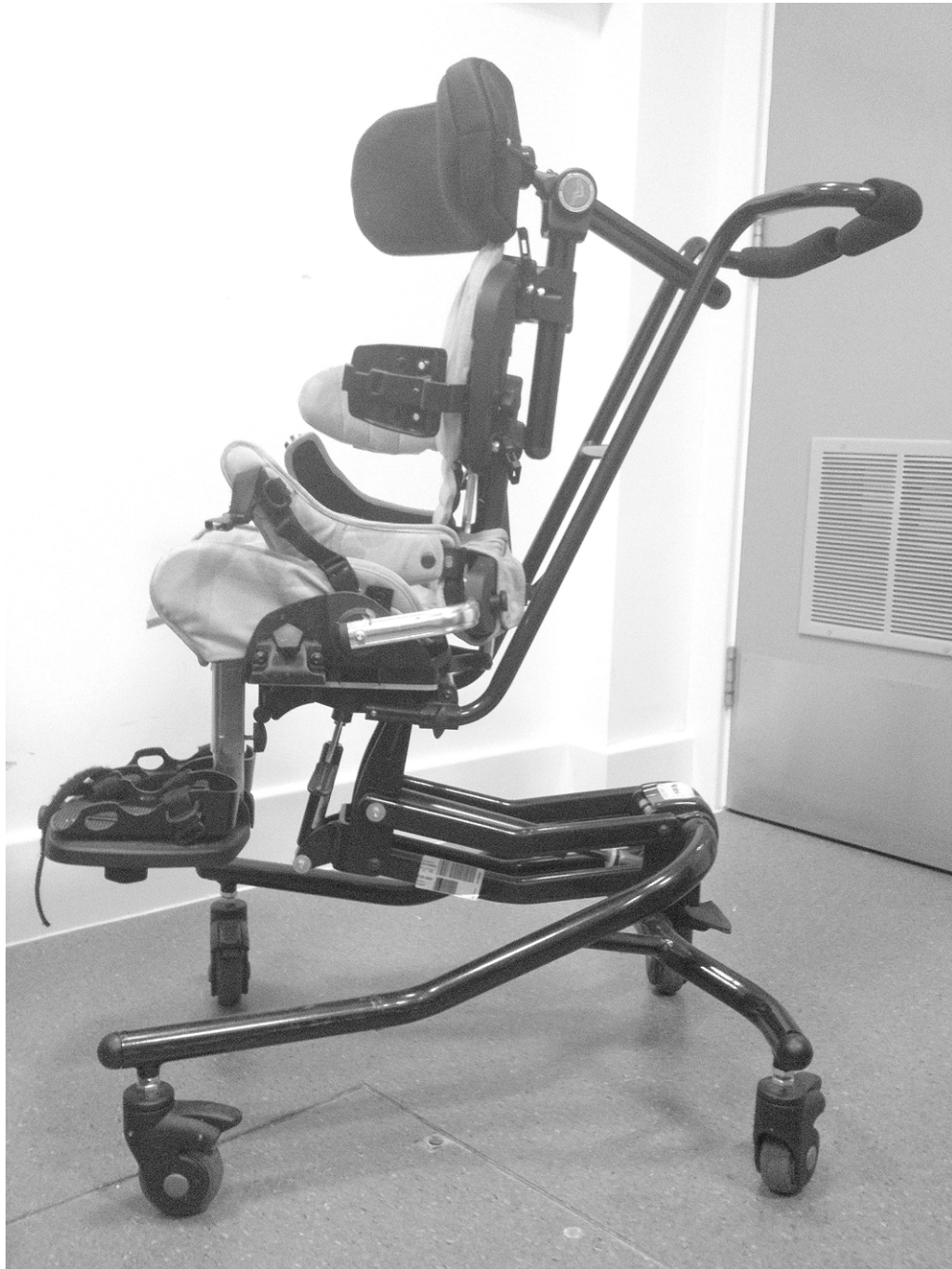
Figure 3-1: A photograph of a commercial rigid seat for disabled children. The photograph shows the usual features on a seat such as this including: Adjustability for size and position, a head support, lateral thoracic supports, a mobile base, adjustable footrest, and lateral hip supports. This seat was used regularly by one of the research participants until it fractured as a result of metal fatigue caused by his powerful extensor spasms.
