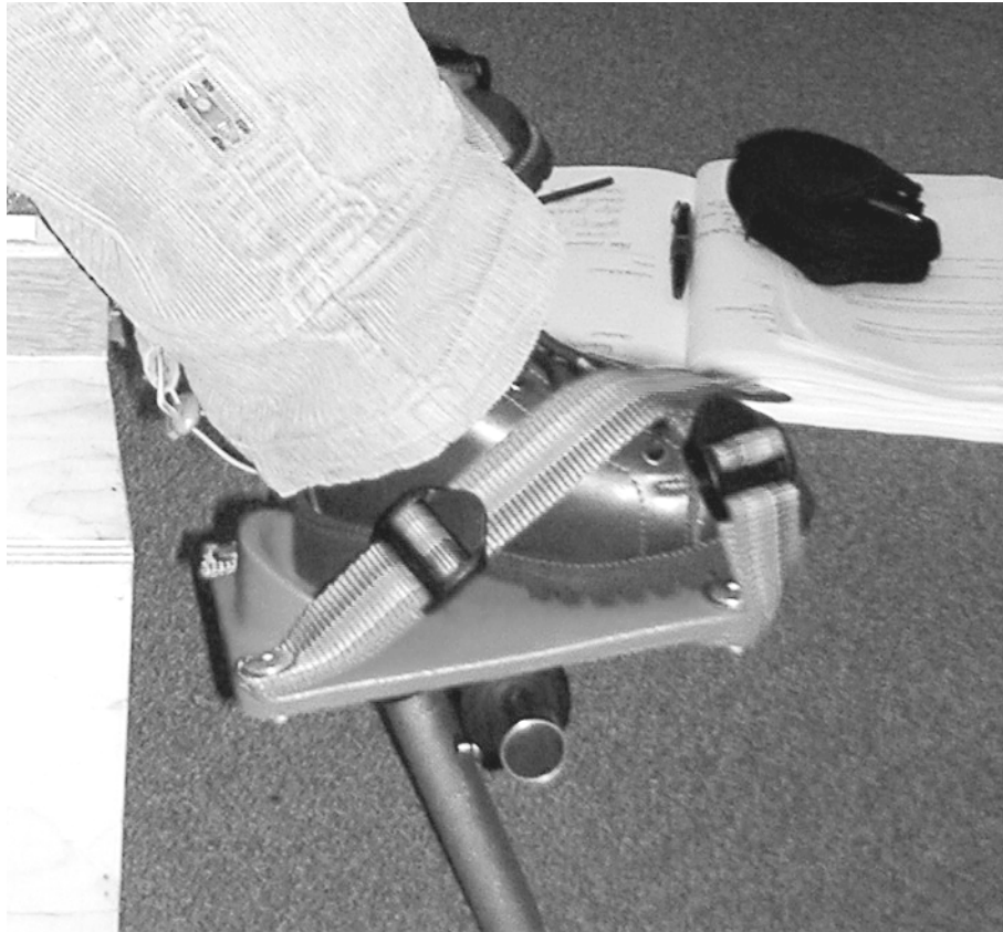
Figure 6-2: A photograph of the foot support on T1's seat, showing the crossed webbing straps running from toe to heel.
