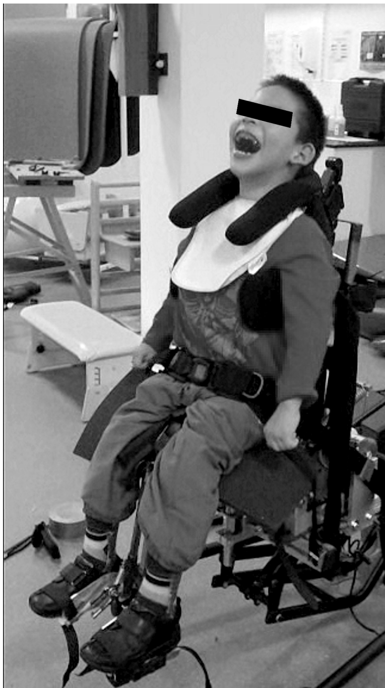
Figure 15-3: A video still of A1 sitting in the second independent seat prototype during the first set-up session on 12 th October 2011. He enjoyed the movement of the backrest and leg supports, and giggled as he moved. The large piece of foam hanging out from the side of the thigh tray has been added to provide additional padding for his thighs, which were impinging on the proximal medial abductive faces of the trays. He sat well, with good head control and active social engagement with the evaluation team.
