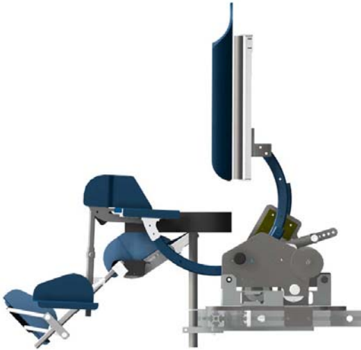
Figure 3a: A drawing of the previous whole body dynamic seat, showing the child's legs in flexed and partially extended positions.
