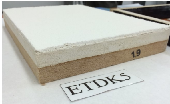
Figure 3.4 Photocatalytic lime mortar ETDK5 – Chapter 7.
