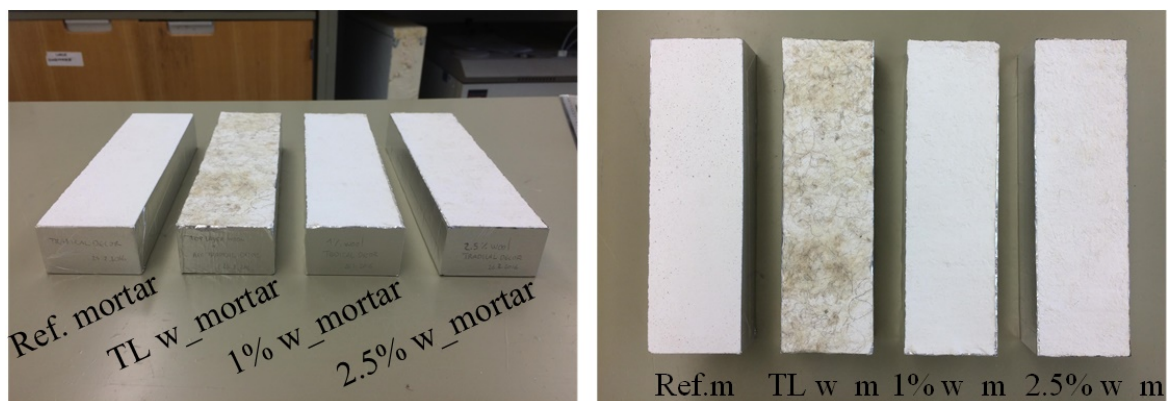
Figure 6.3 Photographs of the lime mortars with different amounts of natural wool added.
