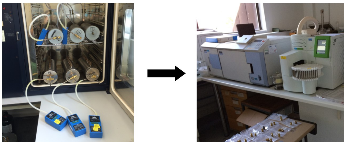
Figure 3.22 Sampling of VOCs and analysis by GC-MS/FID.
