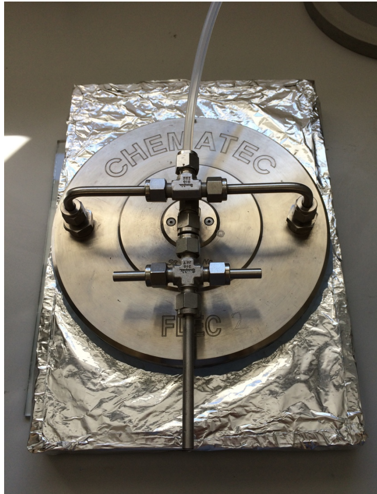
Figure 3.20 FLEC on top of the sample of H2 clay plaster covered with aluminium foil on that part of the sample surface not being tested.
