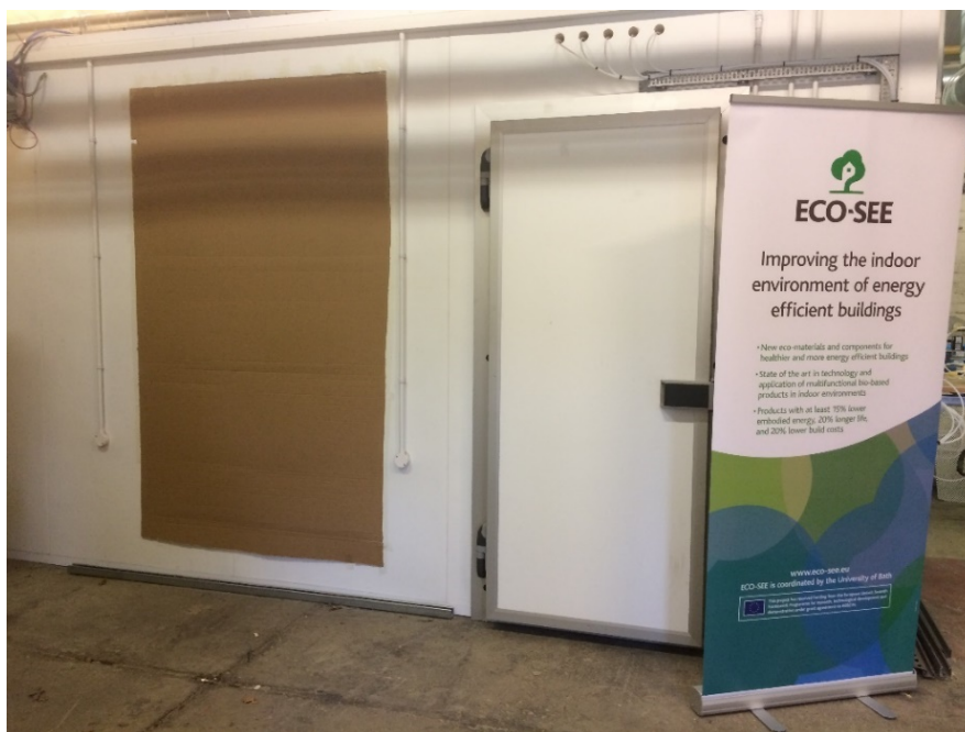
Figure 7.4 30 \text{ m}^3 chamber with the window covered for IAQ assessment under dark conditions.
