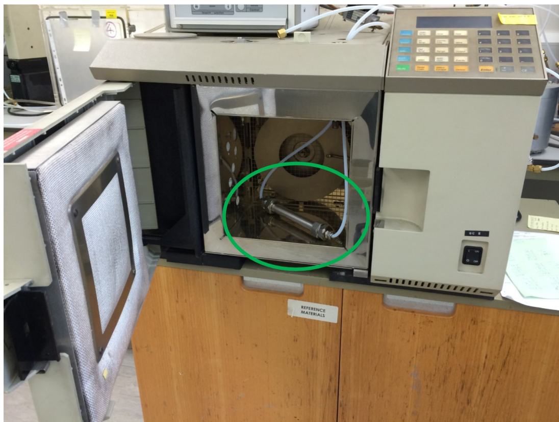
Figure 3.13 Source of formaldehyde KIN-TEK TM inside the oven at 80 °C, to give a stable emission rate.
