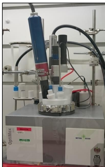
Figure 4.11: Mettler Toledo OptiMax with inline process monitoring using a Raman PhAT probe and FBRM probe
