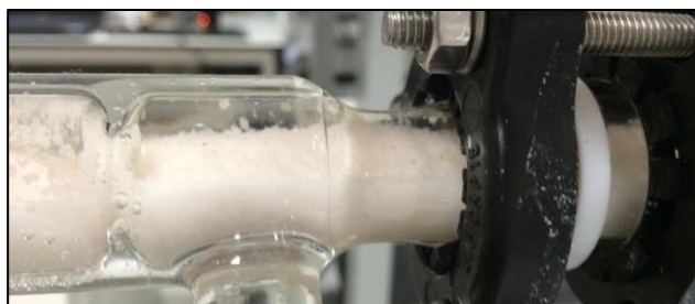
Figure 5.17: High solid loadings in Experiment COBC 9
