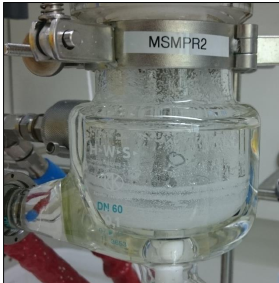
Figure 4.22: Encrustation on the walls of MSMPR 2 in experiments AZ2 and AZ3.
