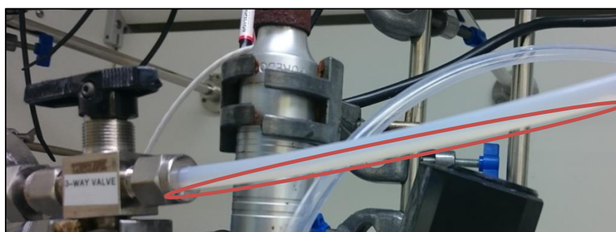
Figure 4.18: Settling of solid in vacuum transfer lines
