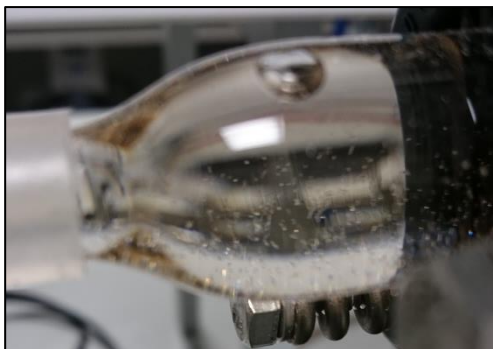
Figure 5.5: Crystallisation in the exit piece in experiment COBC 3
