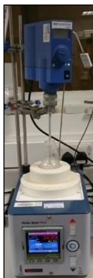
Figure 4.2: Polar Bear Crystalliser with overhead motor and shaft to provide overhead stirring to the system
