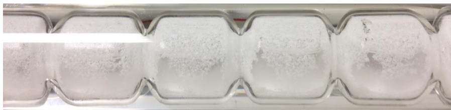
Figure 5.4: Encrustation on the baffle walls in Experiment COBC 1
