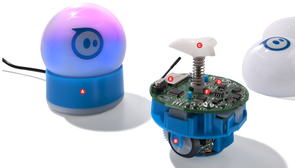
Figure 3-5: Sphero 2.0 robot's internal configuration. Adapted from [56].
