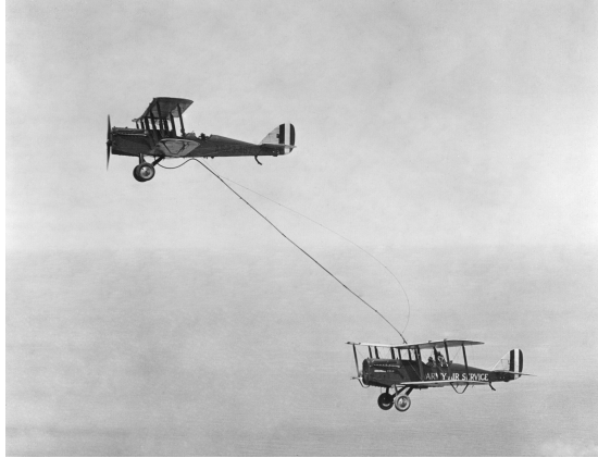
Figure 1.1: Early AAR manoeuvre performed by Capt. Lowell H. Smith and Lt. John P. Richter, at Rockwell Field, California, June 1923. They stayed in the air four days using DeHaviland airplanes. (U.S. Air Force photo) [6]
