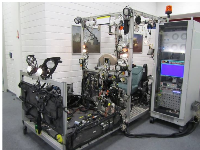
Figure 2.3: Test bench at AGCO Fendt using combined HiL and SiL to test electronic control units and peripheral electronics of a tractor. (Speedgoat GmbH) [46].
